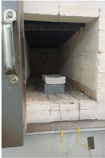
Figure 3.4. The inside of a programmable furnace with an ingot (bottom) and dummy (top) sandwiching thermocouples.
