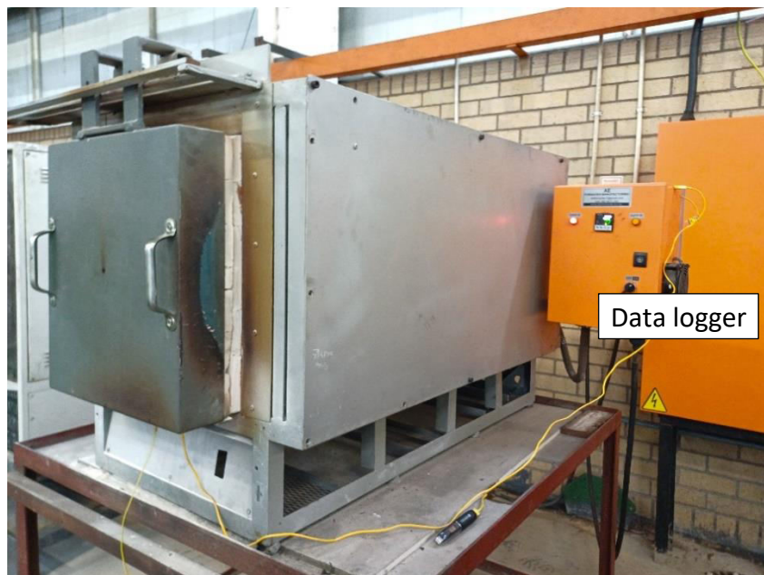
Figure 3.3. Programmable furnace with a thermocouple connected to a data logger.
