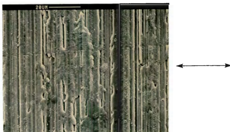
FIGURE 6.10 : Polymer transfer on the counterface of a specimen from a 0,25 \text{ m.s}^{-1} test in water. The arrow indicates the sliding direction
