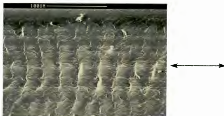
FIGURE 6.9 : Adhesive wear of the polymer surface from a test in water at 0,5 m.s -1 . The arrow indicates the sliding direction
