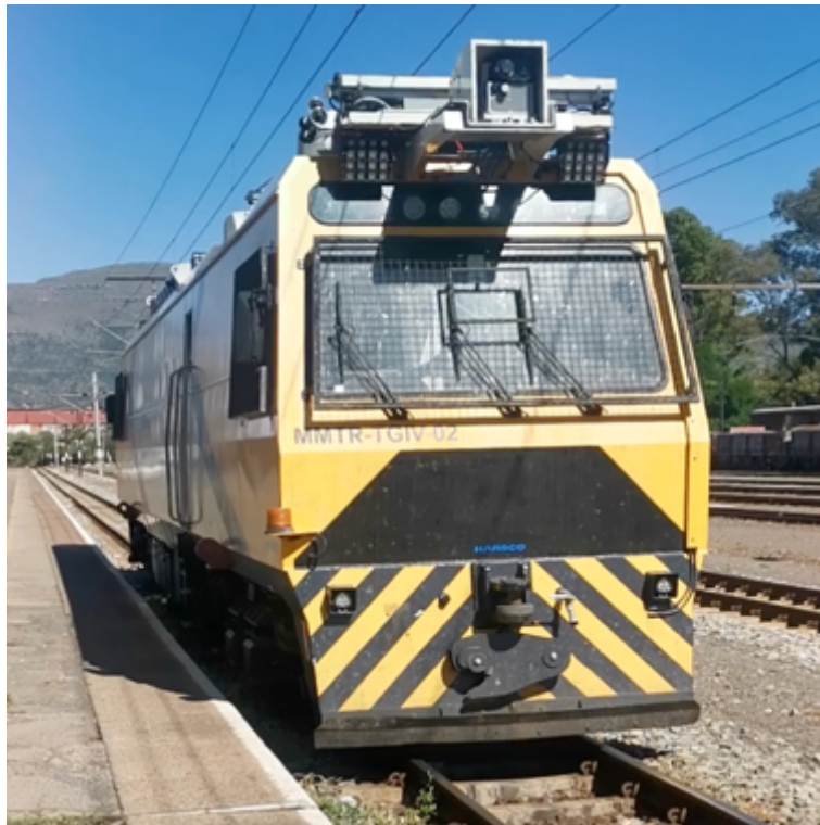
Figure 2-38: Infrastructure Measuring Vehicle near Queenstown (TGIV) (Photo by Author)
