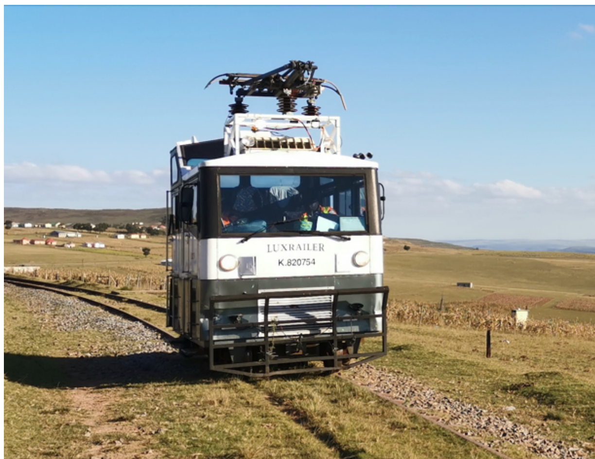
Figure 2-31: LuxRailer Inspection Trolley (Photo by Author)
