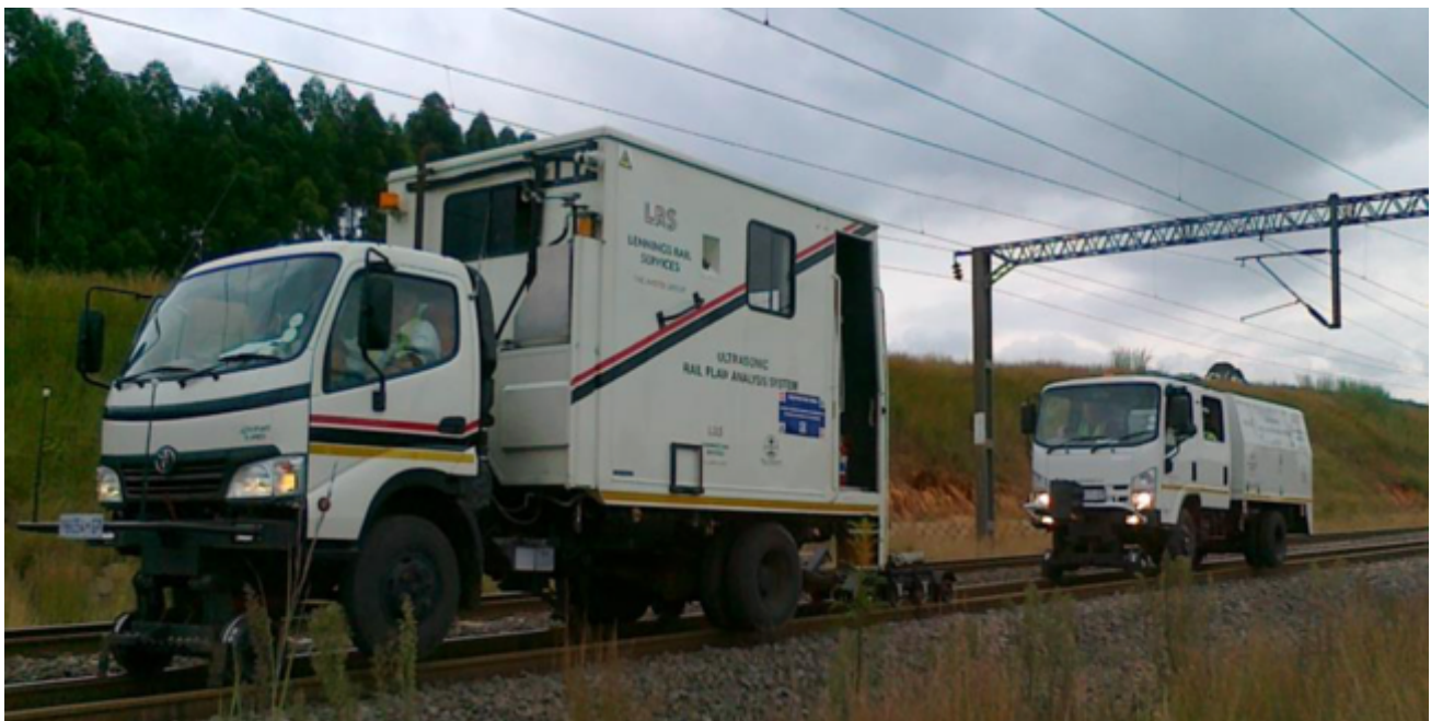
Figure 2-37: Ultrasonic Rail Testing Vehicle and Chaser (Lennings Rail, 2020)
