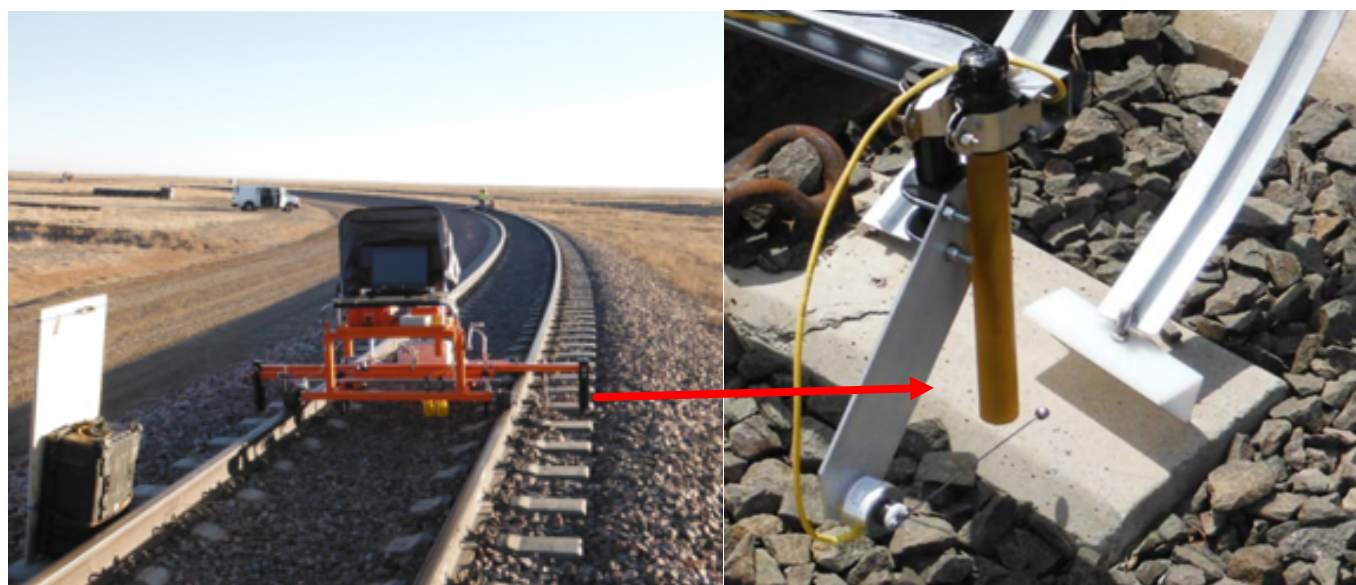
Figure 2-35: Ultrasonic Rail-Mounted Sleeper Assessment, Left; Ball-end tapper Inducing Pulse on Sleeper End, Right (Federal Railroad Administration, 2018)
