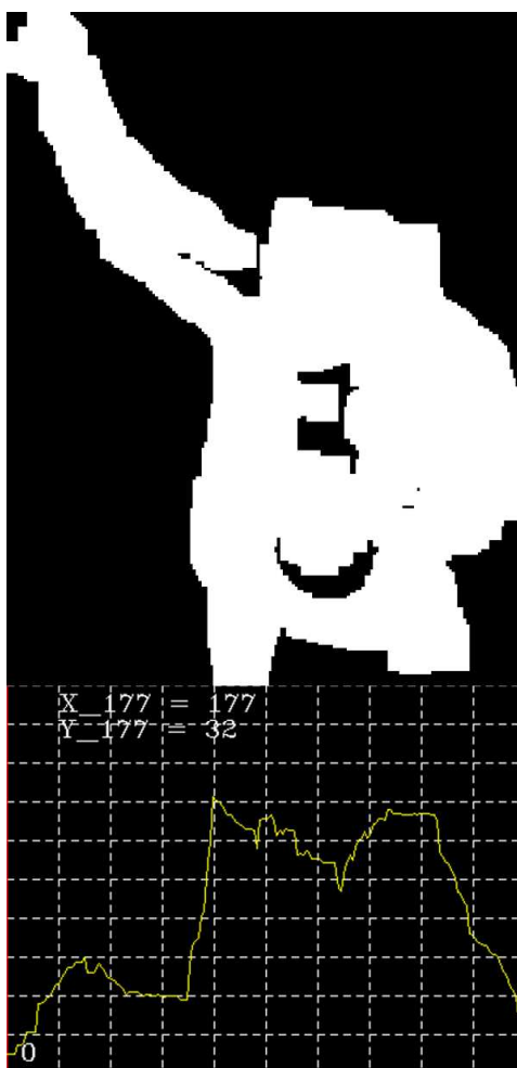
Figure 3.14.: The number of white pixels is summed per column and displayed in a line graph. A signal processing algorithm to detect the step could be used to calculate a specific partitioning line which separates the gesture from the body more accurately than the approximation approach of partitioning the box into halves.
