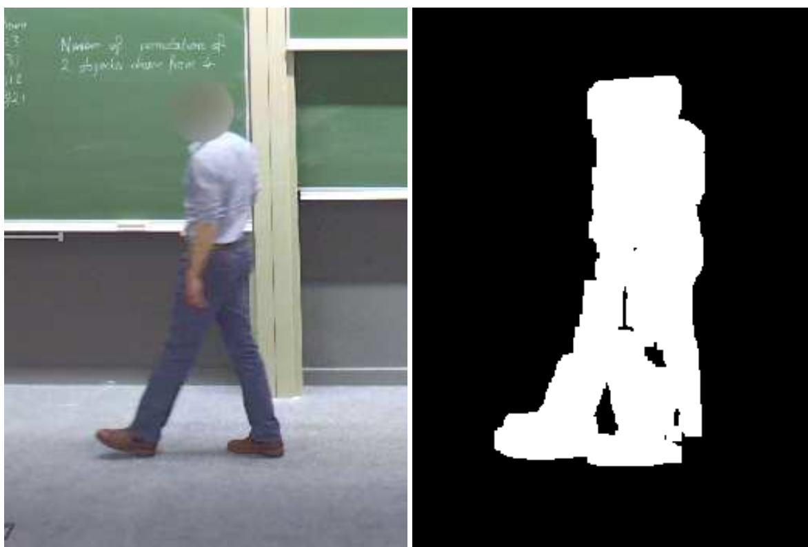
Figure 3.15.: Example of a false positive gesture if only the halves are considered. Checking to ensure that the top quadrant has more white pixels than the bottom avoids this problem.
