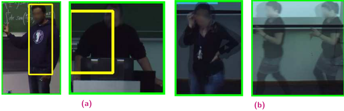
Figure 4.7.: (a) Example of IOU = 0.3 between ground truth (green) and system (yellow) detections. (b) Examples of “low” and “high” presenter motion, respectively.
