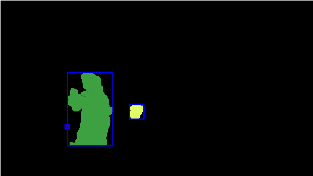
Figure 3.6.: Connected component analysis showing three separate blobs with different colours. The green region represents the presenter, while the presenter's shadow causes the other two blobs. The bounding boxes shown here are created after performing the CCA.
