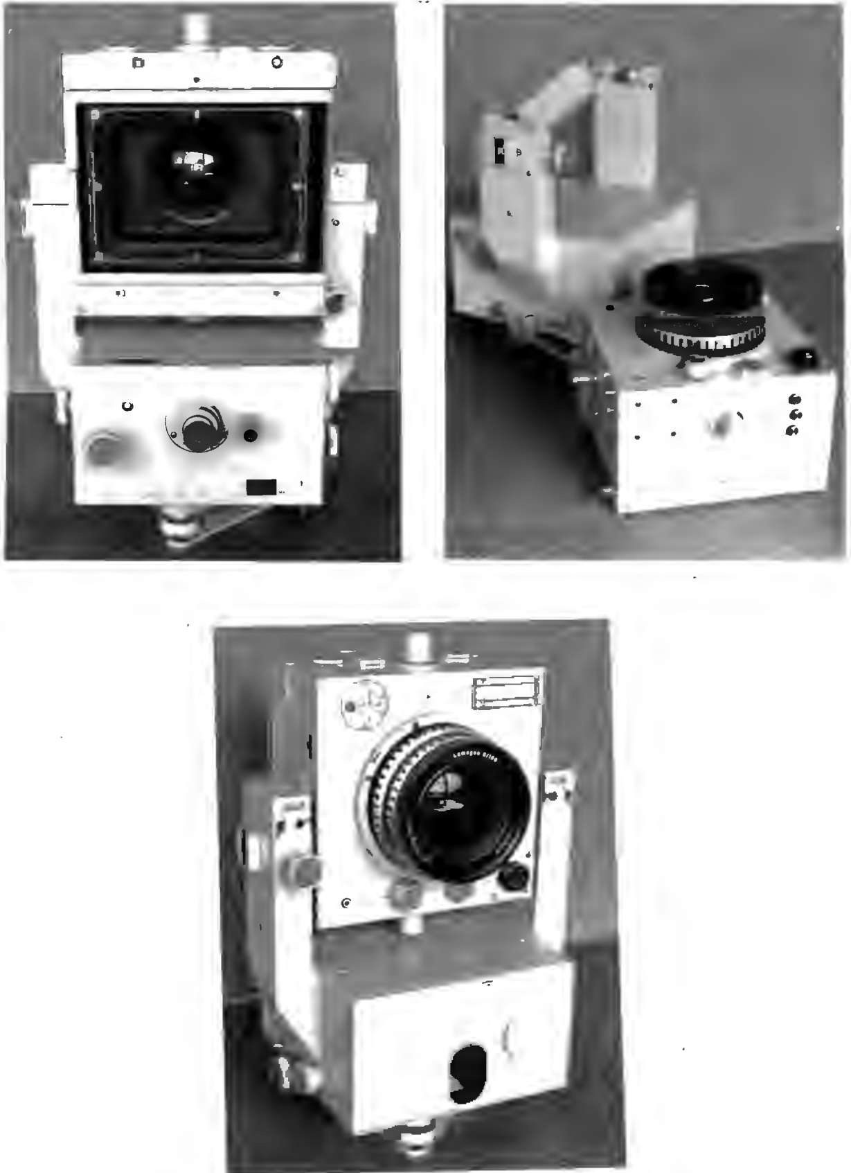
Fig. 4-6 Views of a UMK 10/1318 camera showing the camera with its theodolite mounting, the fiducial marks and the axis studs.
