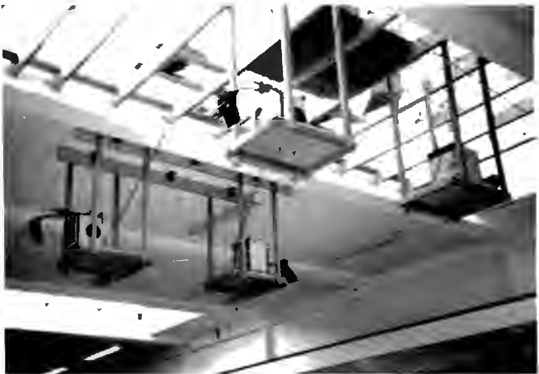
Fig. 4-19 Projector platforms above wave basin.
