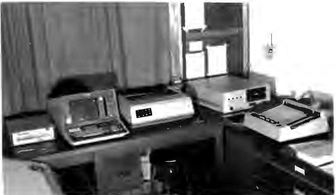
Fig. 4-9 Tektronix microcomputer system consisting of (from left to right) digitiser tablet and digitiser control unit, central processing unit with VDU, line printer, file manager and plotter.
