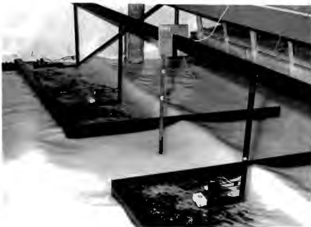
Fig. 5-8 Wave probe used to measure incident wave height.
