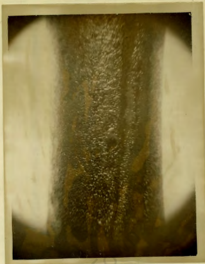
Plate 21. Sulphur Dioxide Type of Corrosion. x 2
