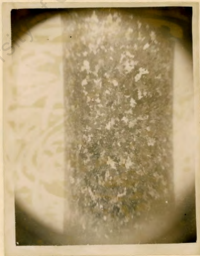
Plate 12. Coarse-Grained Structure. x 2
