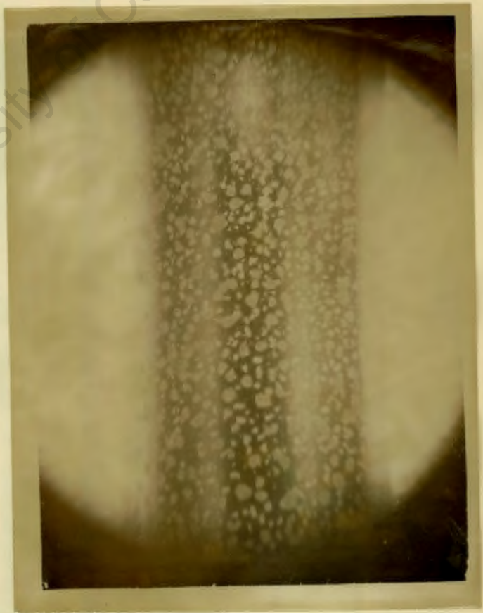
Plate 14. Corrosion Pit Holes. x 2
