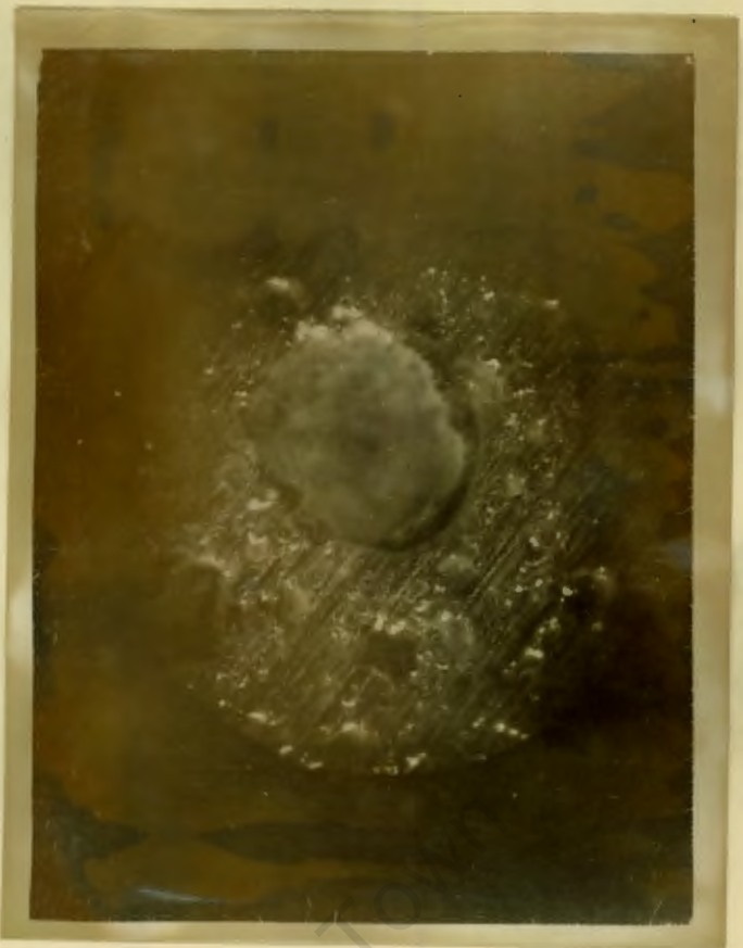
Plate 17. 2-hour Corrosion Spot. x 160
