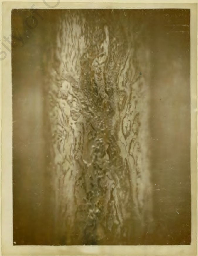
Plate 4. Streaky Corroded Test Specimen.
