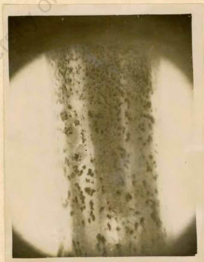
Plate 9. Band at End of Heat-treated Test Specimen. x 2
