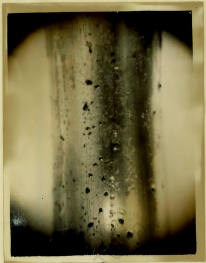
Plate 26. Pitting Attack by Vapours of Ammonium Nitrate. x 2
