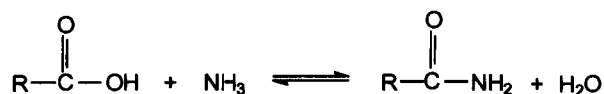
Figure 2.3: The formation of an amide bond through the amidation of a carboxylic acid with ammonia.
