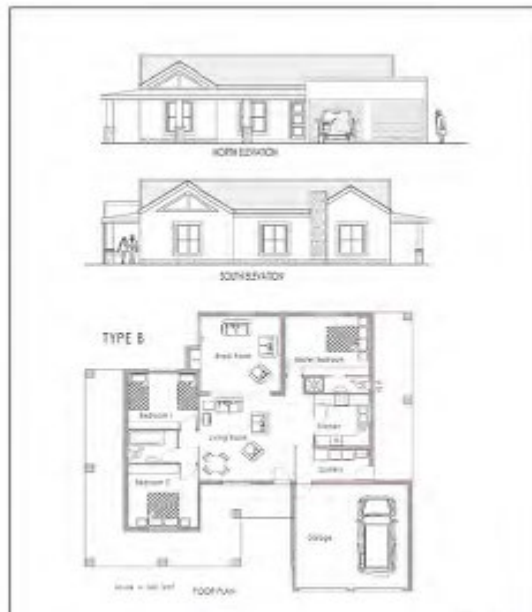
Figure 7.4: Preliminary Design Drawing and Floor Plan of a Single House at a Golf Course
