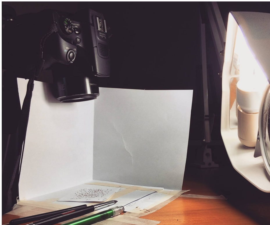
Figure 5.2: A camera set-up above a white paper with E. discolor seeds to ensure that a useable and comparable photograph can be taken.
