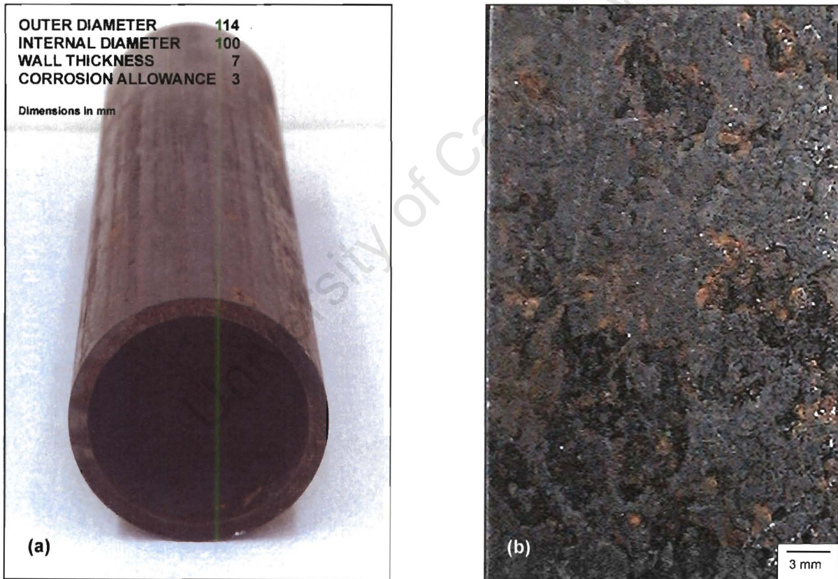
Figure 3-2 (a) Length of unused steam coil tube supplied by PetroSA for testing. (b) Specimen used to test the effect of the original surface on erosion (geometry as in figure 3-1a).
