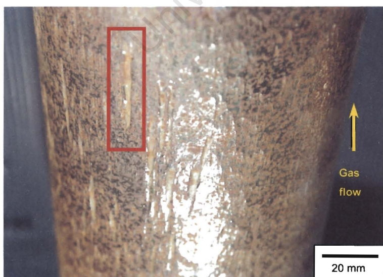
Figure 1-2 Wear damage of the lower end of a heat exchanger tube (steam coil tube) removed from service. Arrows in (a) indicate the orientations of subsequent images.
