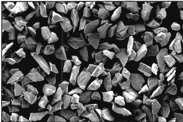
Figure 4-6 Morphology of erodent particles used in erosion tests: (a) Fresh (milled) catalyst, (b) spent catalyst and (c) silica particles.
