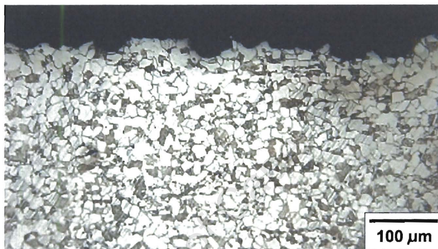
Figure 4-24 (20X) Cross-section of surface of plasma nitrided tube steel
