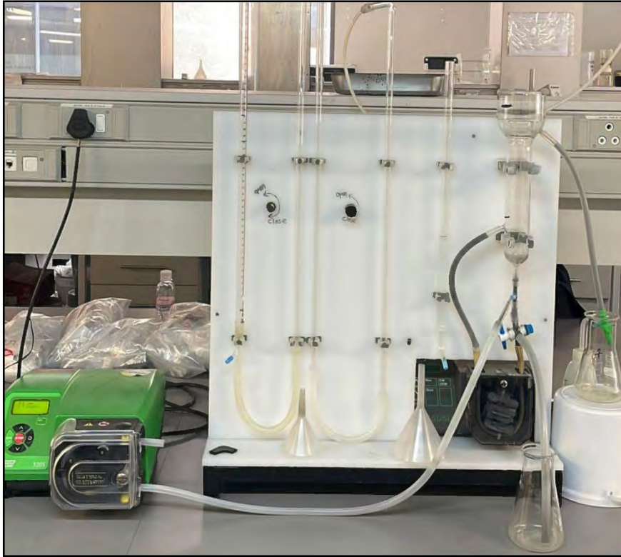
Figure 3.14: UCT microflotation rig used in this study
