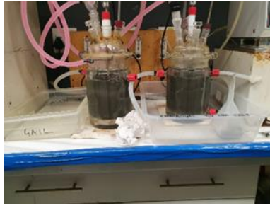
Figure 4.1: Photograph of BRGM-KCC stock cultures used for Microwell plate tests and to inoculate bioreactors
