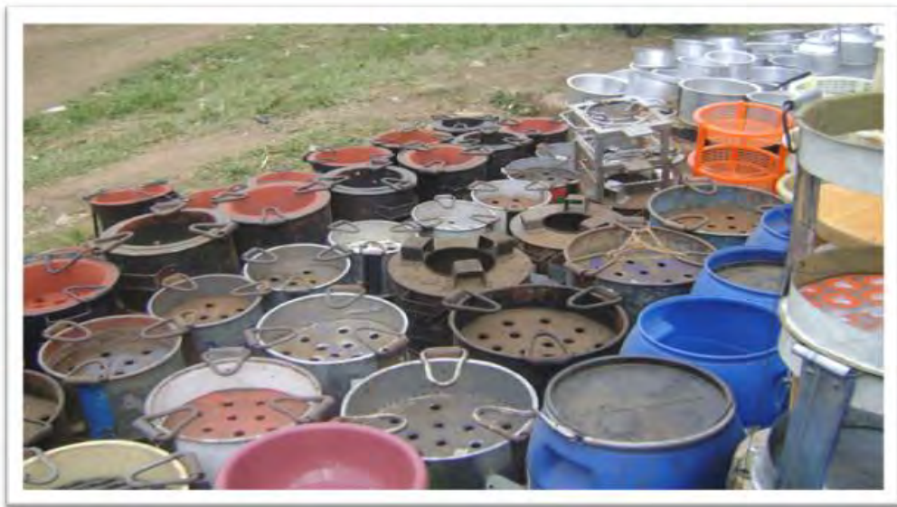
Diagram 4.7 'Jiko' basic model and improved clay insulated charcoal stove
