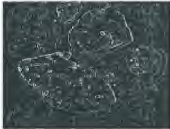
Figure 3.8: The Sobel operator output obtained using a neighborhood size of 3x3
