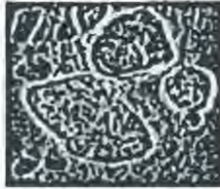
Figure 3.11: The Laplacian of Gaussian operator output with a neighborhood size of 4 \times 4 and a sigma value of 2.5
