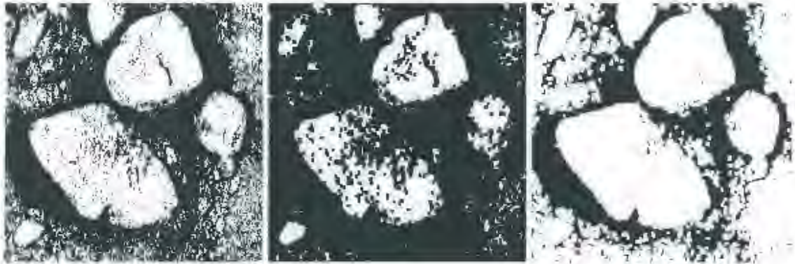
Figure 5.2: The original binary image, binary eroded and dilated images with a square structuring element of size 3 \times 3 . The original sample image is adaptively thresholded with a window size of 91 \times 91 .
