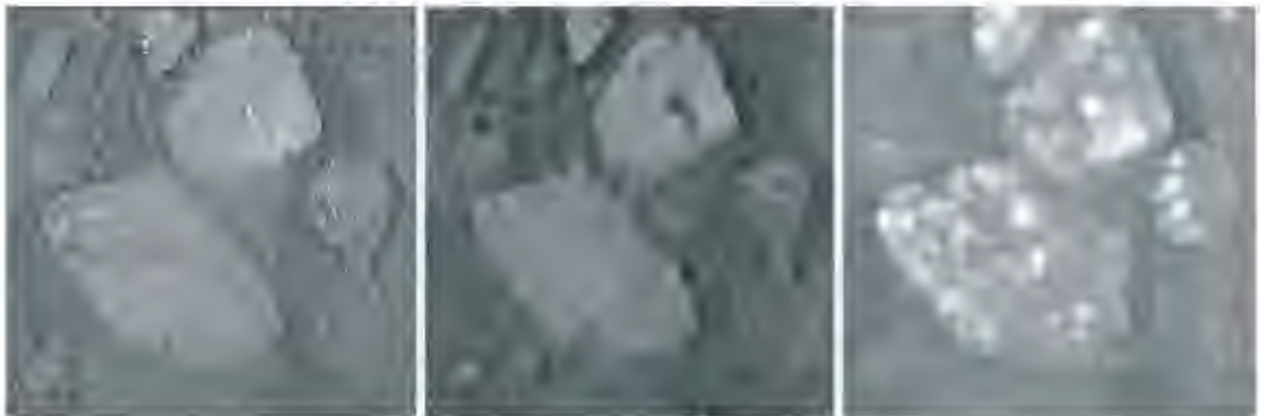
Figure 5.3: The sample image, grayscale eroded and dilated images with a disk structuring element of radius 5.
