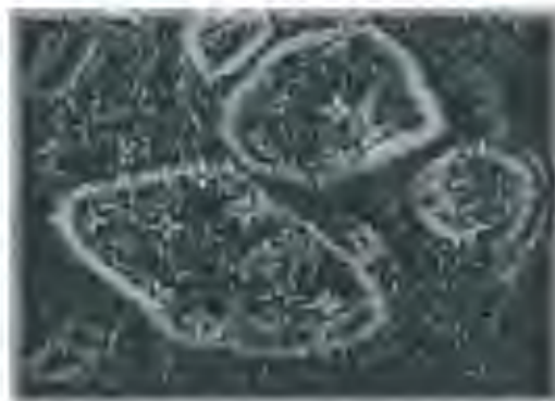
Figure 3.13: The Canny operator output with a sigma value of 2.5
