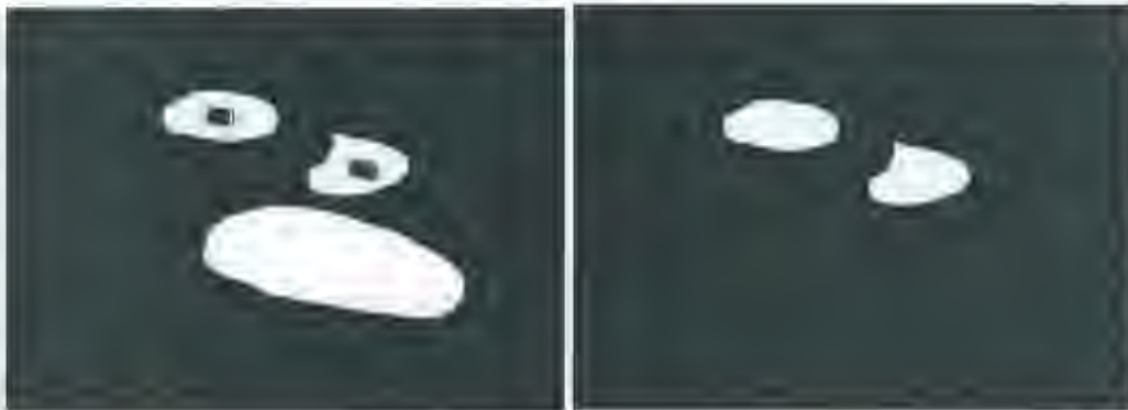
Figure 5.9: Binary reconstruction of the white areas with the black areas within the white blobs as the set of markers.
