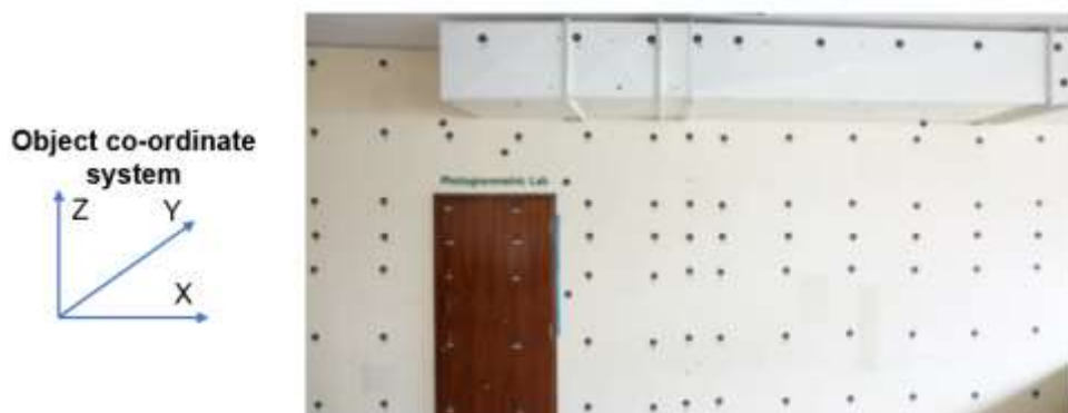
Figure 3-1 Calibration testfield at University of Cape Town
