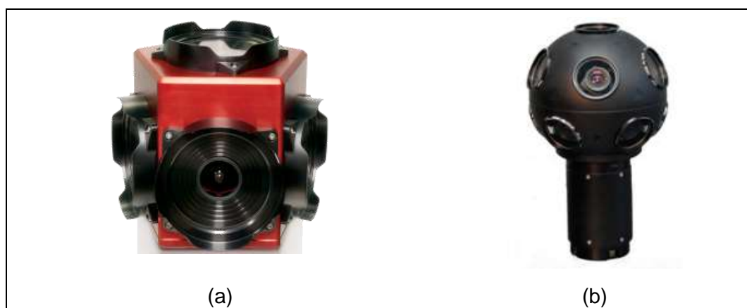
Figure 2-4 Multi-head panoramic cameras: (a) Ladybug 5 (Pointgrey, 2015) (b) Dodeca 2360 (Agarwal, 2007)
