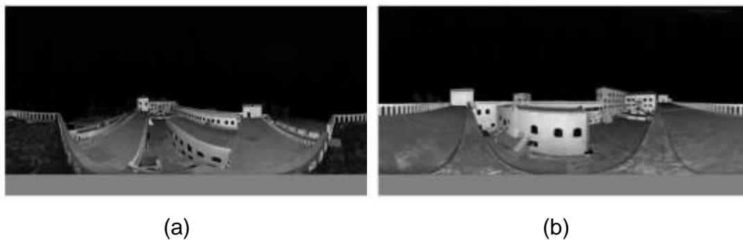
Figure 6-4 Panoramic intensity images of Elmina castle used for the laser scan registration
