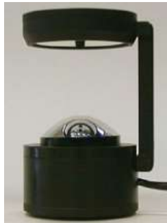
Figure 2-2 Catadioptric camera system with a hemispherical FOV (Nayar, 2001)
