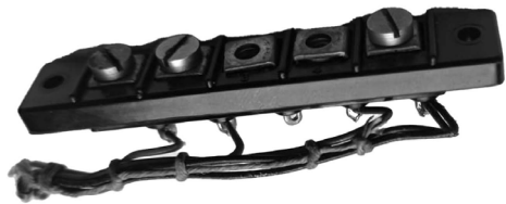
FIG 12. Melissa Wrench, Terminal with missing screws . 2023.
