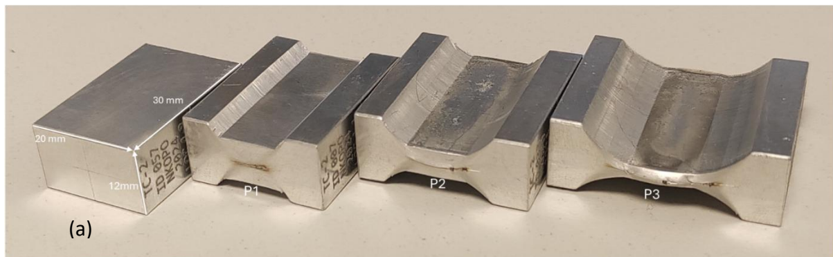
Figure 12 Samples used for PSC tests (a) before deformation (P1, P2, and P3) after deformation pass 1, 2 and 3, respectively.
