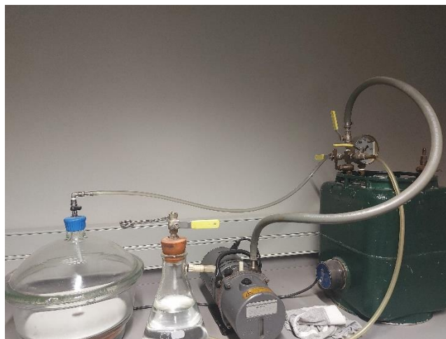
Figure 3-2: Vacuum apparatus for specific gravity
