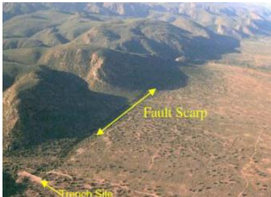
Figure 2-8: The Kango fault showing part of an 84 km long and 2m high fault scarp produced by an Mw 7.4 event about 10600 years ago (Midzi & Goedhart, 2009)
