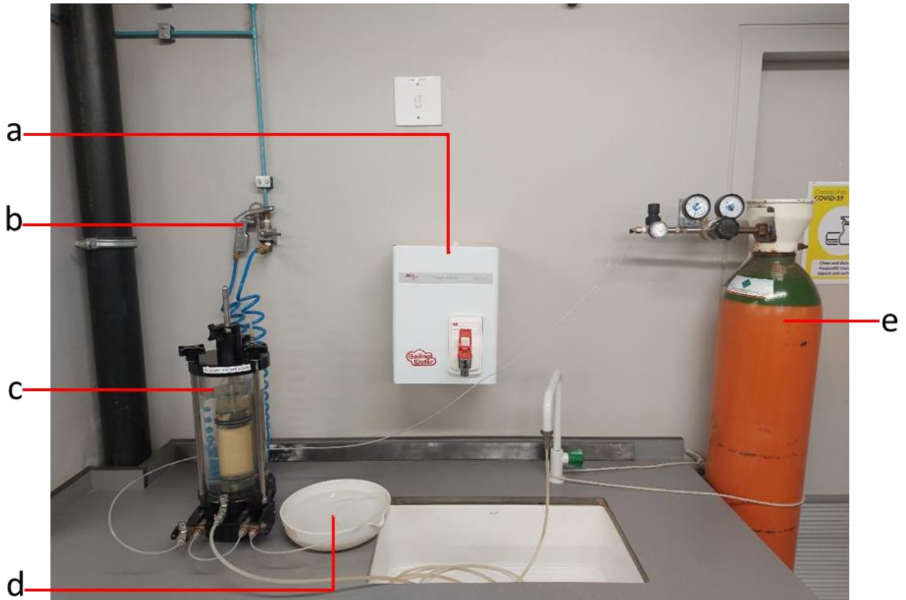
Figure 3-6: Set up for pre-saturation with carbon dioxide
