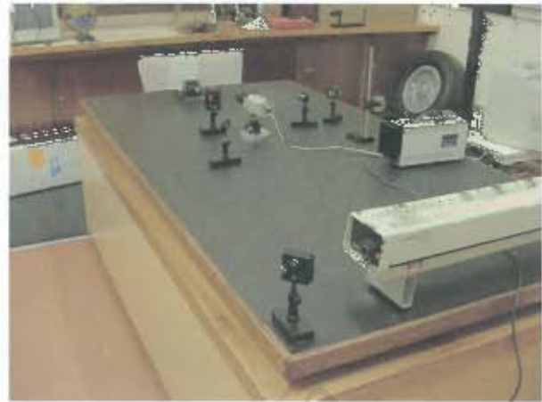
Figure 2.2 ESPI vibration isolation table at UCT
