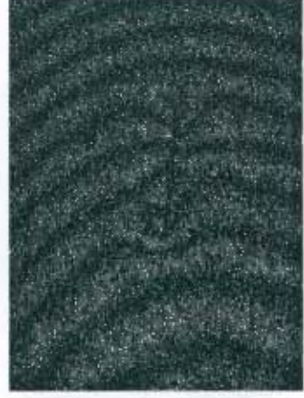
Figure 5.23(a)-(e) ESPI images of test specimen exposed to environmental excitation captured using electronic shutter (camera shutter) at exposure times of 20ms, 8.33ms, 2ms, 0.5ms, and 0.1ms respectively
