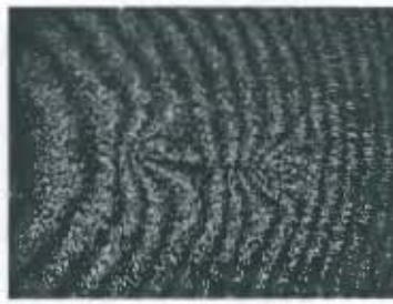
Figure 5.17(a) – (f) ESPI images of test specimen exposed to environmental excitation captured using mechanical shutter (large disc) to pulse laser at exposure times of 20, 5.2, 3.2, 1.9, 0.9 and 0.5ms respectively
