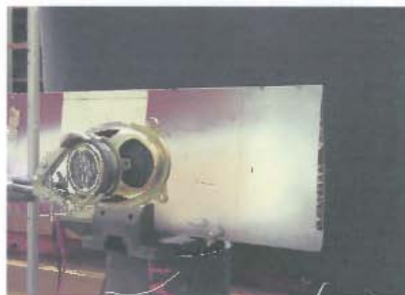
Figure 4.3 Test specimen excited by loudspeaker
