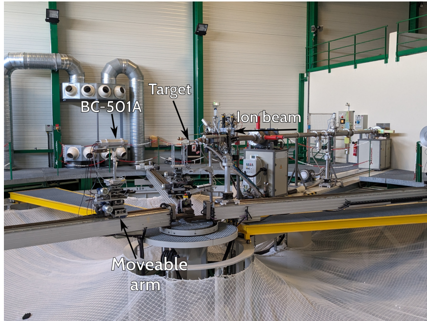
Figure 4.1: The AMANDE experiment hall. Coming from the right is the beamline, which is incident on the target at the centre. Movable arms allow for the placement of detectors anywhere between -160^\circ and +160^\circ to the ion beam, and between 0.5 m and 6.0 m from the target.
