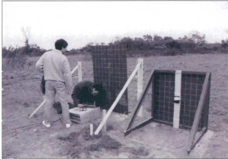
Figure 2.27: Photograph of experimental set up used for air pressure generated from explosive devices [10]
