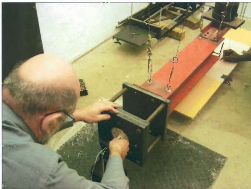
Figure 2.30: Photograph of experimental set up for impulsive loading using plastic explosive mounted directly
