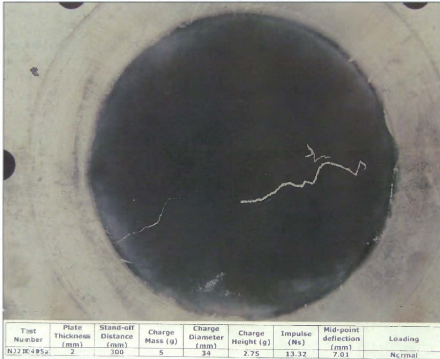
Figure 4.6: Photograph of black soot observed for test plate subjected to load condition LC-1
