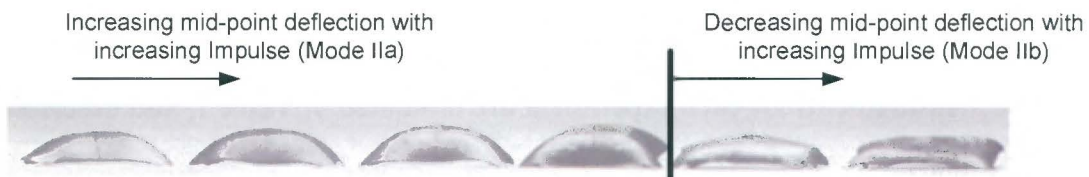
Figure 2.46: Changing mid-point deflection for increasing impulse (uniformly loaded square plates) [4] (repeated figure)
