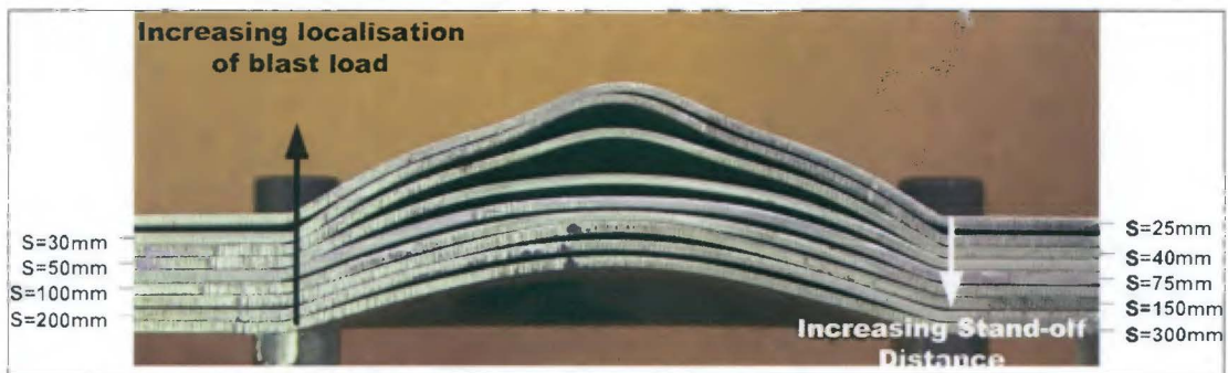
Figure 4.4: Sequential layout of test specimens for increasing stand-off distance for constant charge mass, 7g (Plate numbers top to bottom - NJ160405h, NJ150405b, NJ090405b, NJ020705c, NJ080405b, NJ230405d, NJ050405b and NJ210405d)
