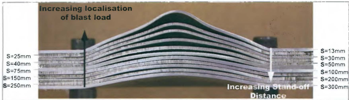
Figure 4.3: Photograph of sequential layout of test specimens for increasing stand-off distance for constant charge mass, 5g (Plate numbers top to bottom - NJ250405b, NJ160405g, NJ160405a, NJ150405a, NJ090405a, NJ020705b, NJ080405a, NJ230405c, NJ050405a, NJ290305f and NJ210405a)
