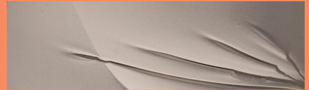
Figure 39 concrete textures replicated from the flexible formwork
