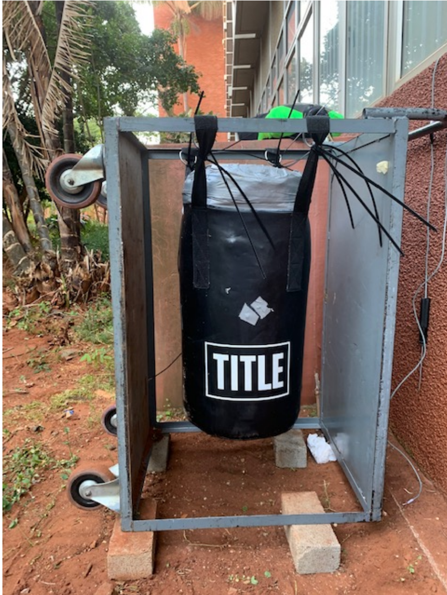
Fig. 8.2 – The cooling dummy suspended during free-air cooling.
