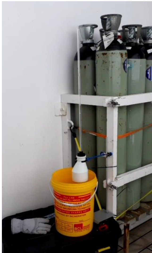
Figure 2.8: Experimental setup of falling head test [75].
