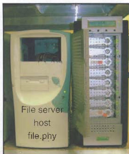
Figure A.5: Photo showing the dedicated file server and RAID array with bay-doors. Red tags denote spare disk and hot-swap disk, for fail-over capability.
