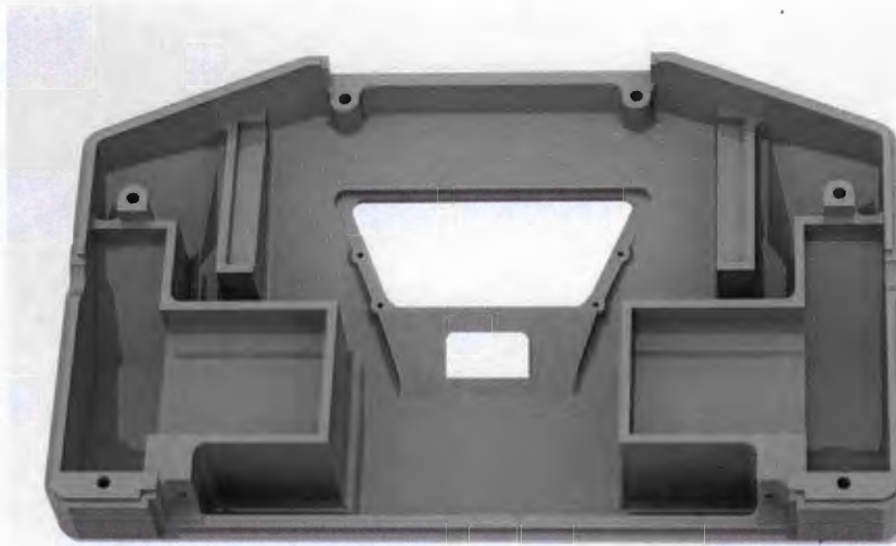
Figure 0.2 The outer shell designed for the robot
