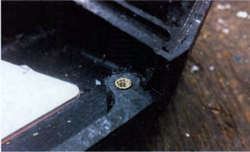
Figure 4.9 Shell with brass thread insert
