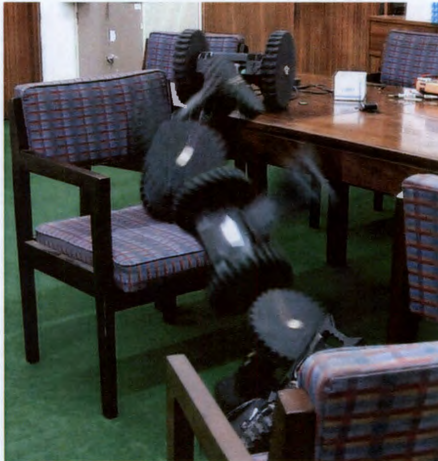
Figure 7.14 Composite im- age showing robot tumbling from one sur- face to another
