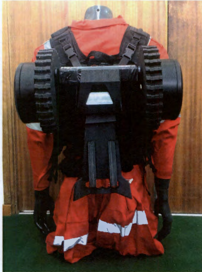
Figure 7.1 The robot stored in the transportation harness
