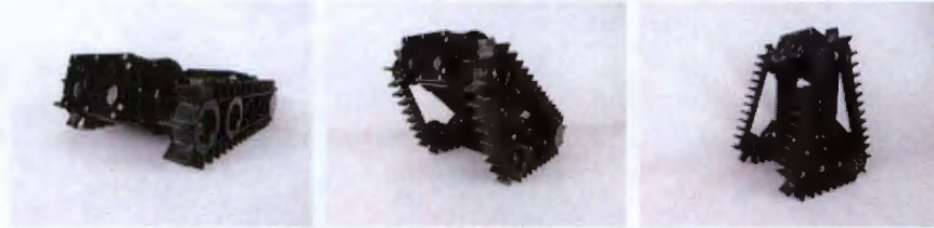
Figure 2.8 The Inuktun VGTV, in three stages of its variable shape[38].
