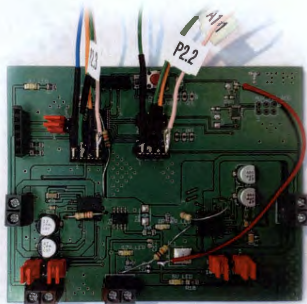
Figure 5.9 The "beta ver- sion" PCB design, show- ing temporary connections to external micro- controller
