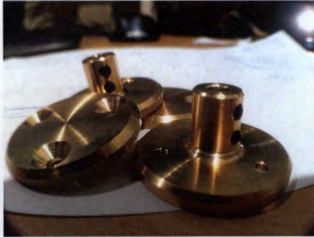
Figure 4.14 The machined brass hubs
