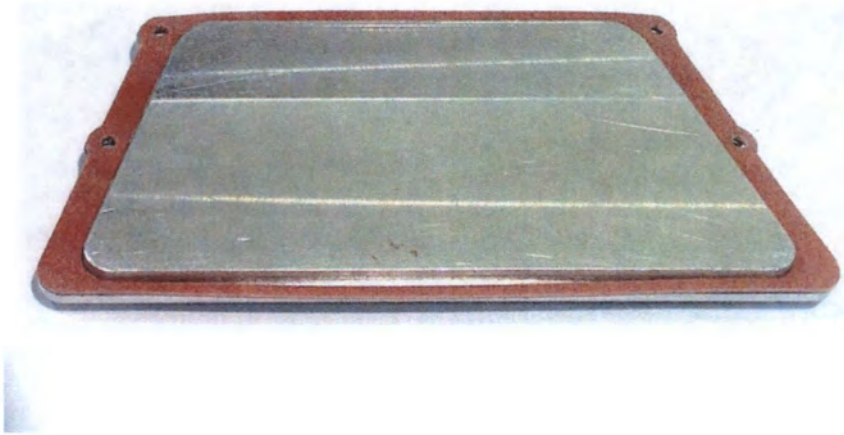
Figure 4.12 0.5 mm silicone seal in position on the heatsink
