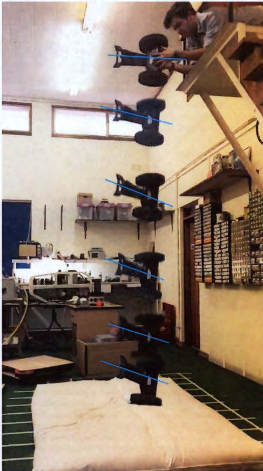
Figure 7.11 Composite image showing yawing effect of tail in drop test
