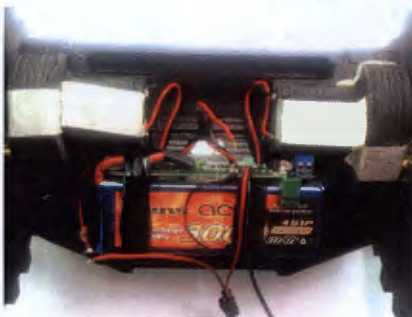
(a) The battery sub-system in position
