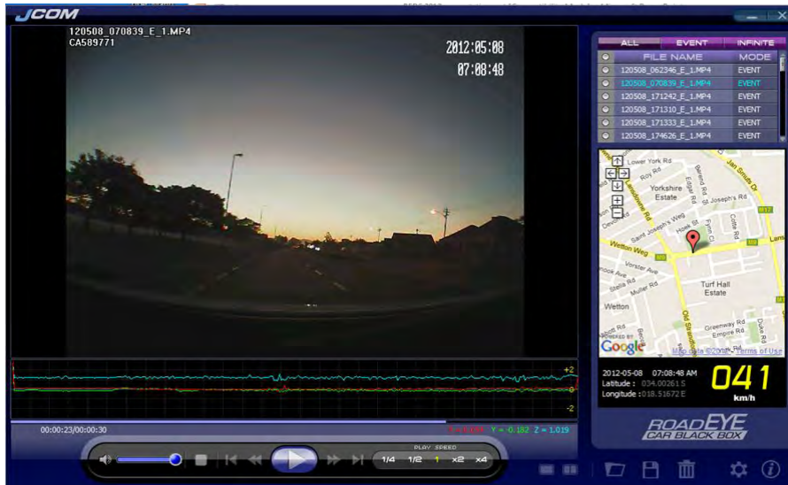
Figure 54: Example of speed and travel time data collection using in-car tracking system
