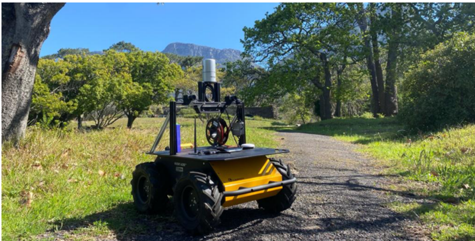
Figure 11.1: Clearpath Husky A200 fitted with sensors used for data collection and testing
