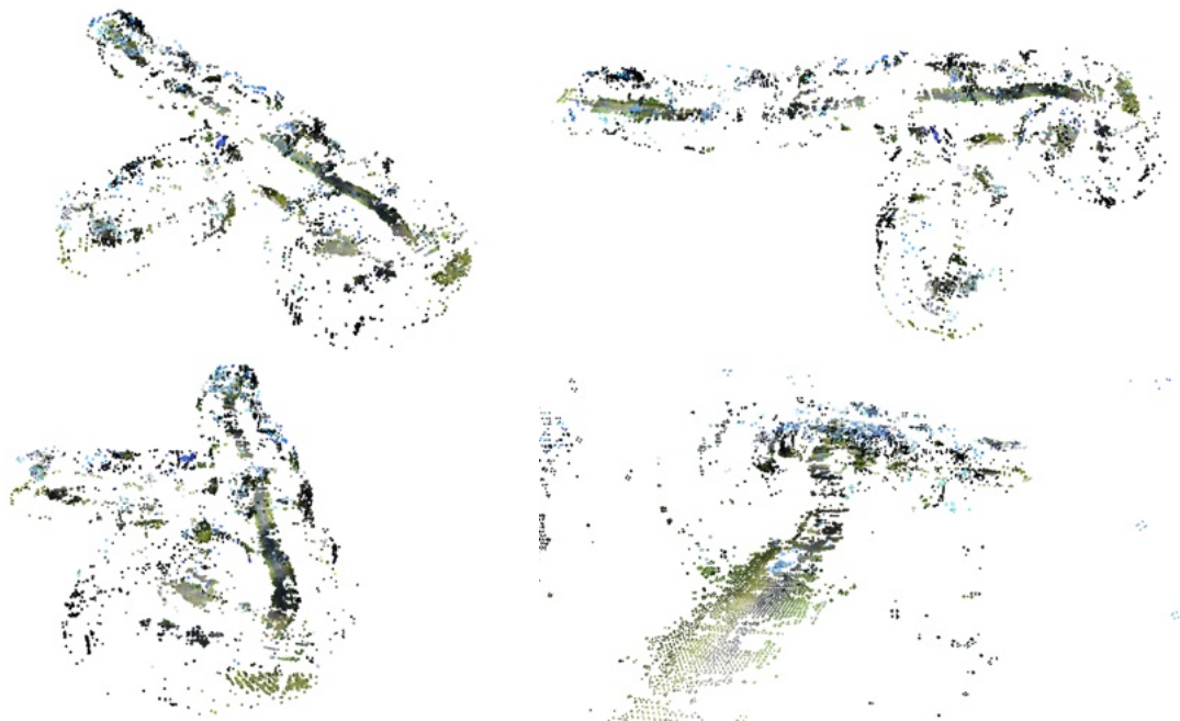
Figure 14.2: Reconstruction on the Zoo using ground truth coordinates and Stereo SGBM as the disparity estimation
