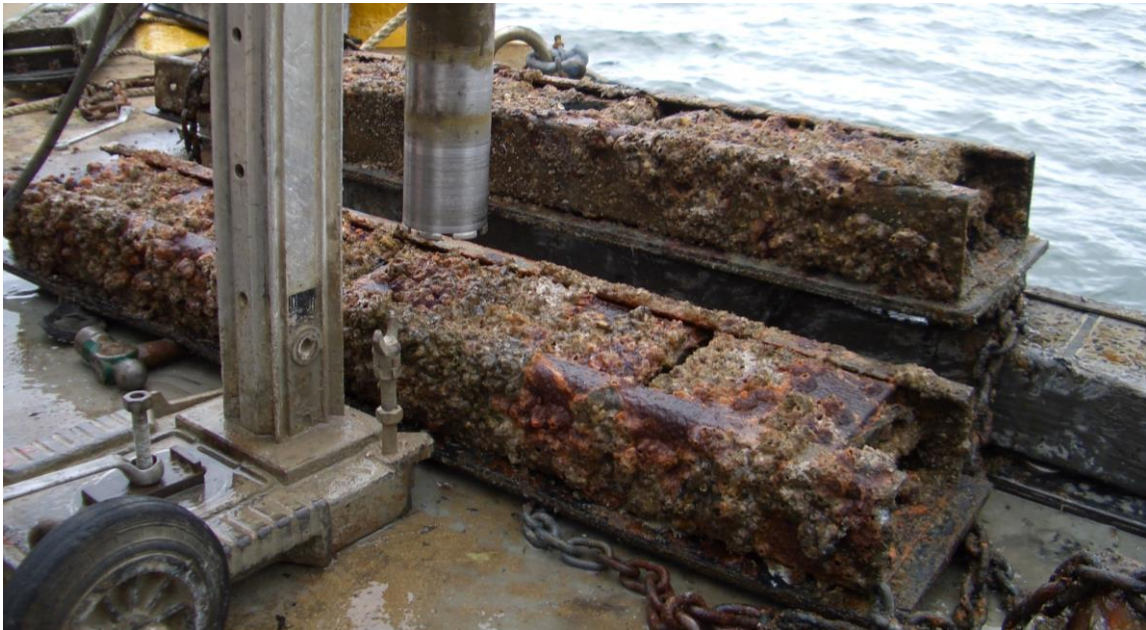
Figure 3.10: Removing of core samples on site (Durban); note the growth of barnacles on the samples (in the submerged zone)
