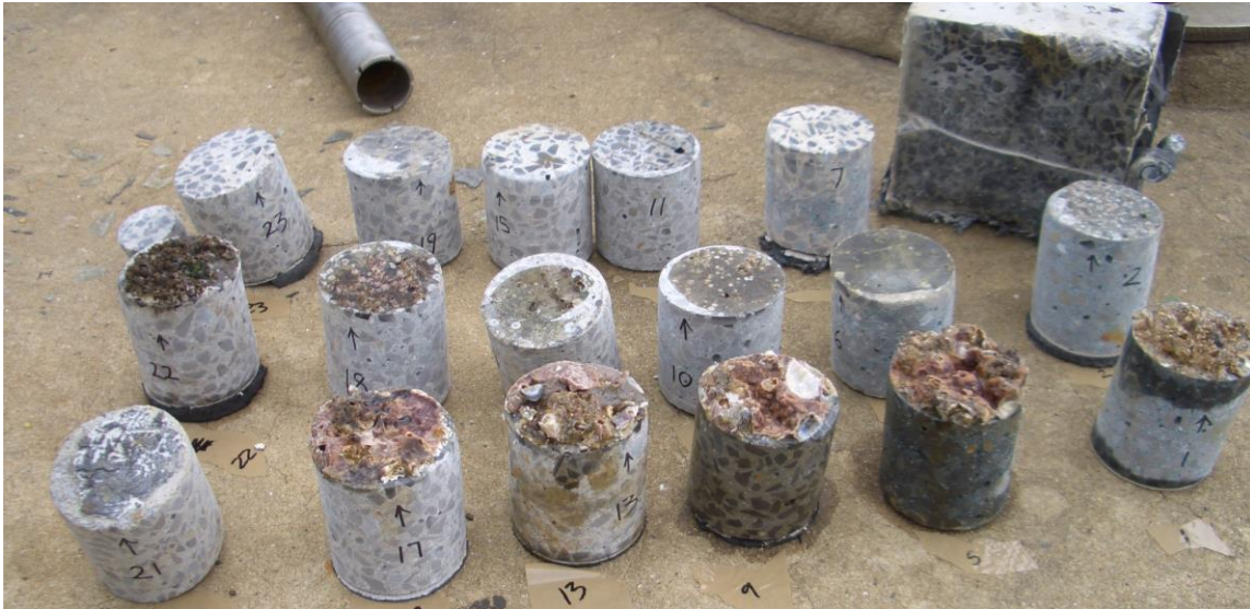
Figure 3.11: Core samples (Durban); bottom row: specimens from submerged zone (with barnacle growth), middle row: splash/spray zone (slightly discoloured), top row: splash/spray zone (“clean” samples”)
