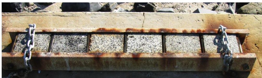
Figure 3.2: Typical site samples in steel frames; per mix and exposure condition, 6 samples were manufactured and placed into a single steel channel frame
