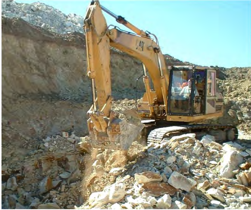
Photo 2 : Mining of the Heidelberg Raw Bentonite
