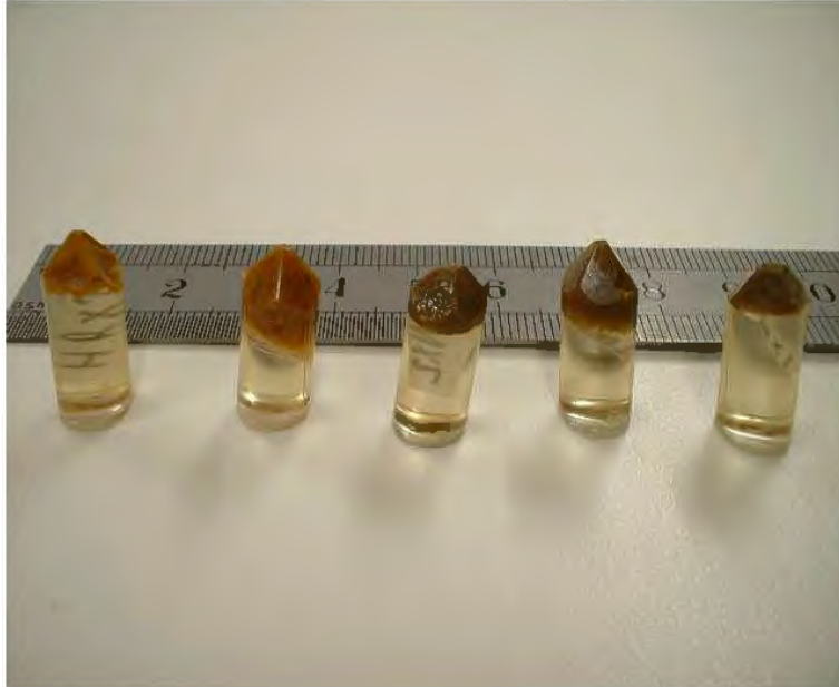
Photo 6: Envirobent and Heidelberg Raw Bentonite samples embedded in resin
