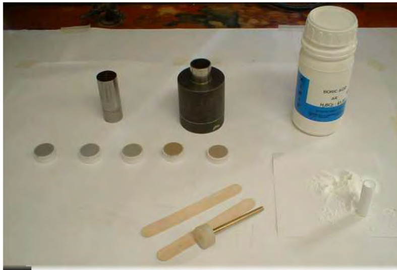
Photo 5: Preparation of Briquette for X-Ray Fluorescence Analysis
