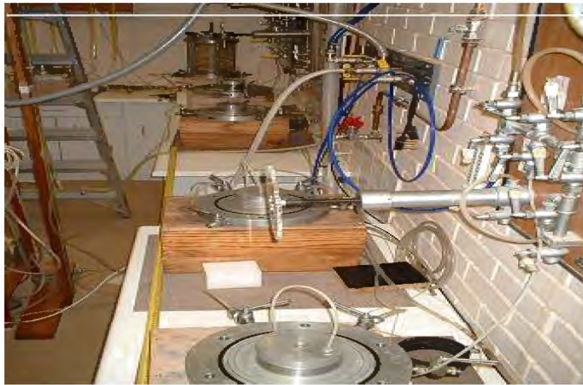
Photo 12: Falling Head Permeability test apparatus
