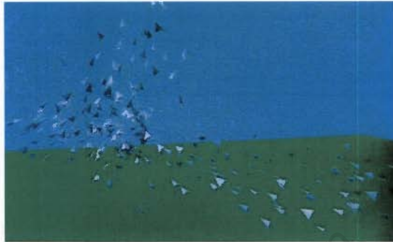
Figure 2.3: The flocking birds created by Reynolds. Each particle is able to exert steering forces in order to avoid collisions and maintain its position in the flock. Image source: [Rey87]
