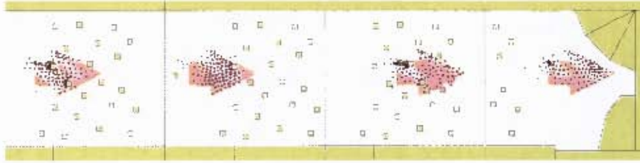
Figure 2.5: The crowd shape control introduced by Chang and Li which has the agents in a crowd attempt to stay within the boundaries of a specified shape. This control is reliant on an agent's ability to stay within the shape and so is somewhat unreliable. Image source: [CL08]
