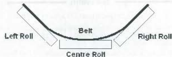
Figure 4.4: The Carrier Idler Arrangement in the Conveyor Belt
