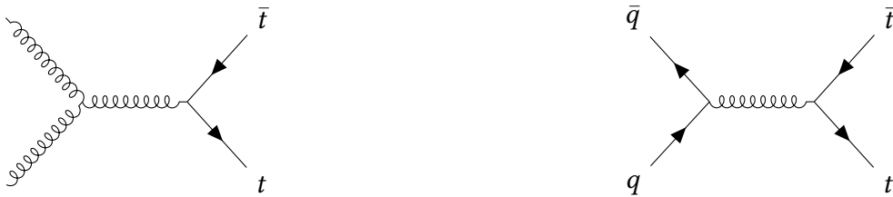
Figure 3.1: Examples of leading order Feynman diagrams for top quark pair production through gg \rightarrow t\bar{t} and q\bar{q} \rightarrow t\bar{t} .
