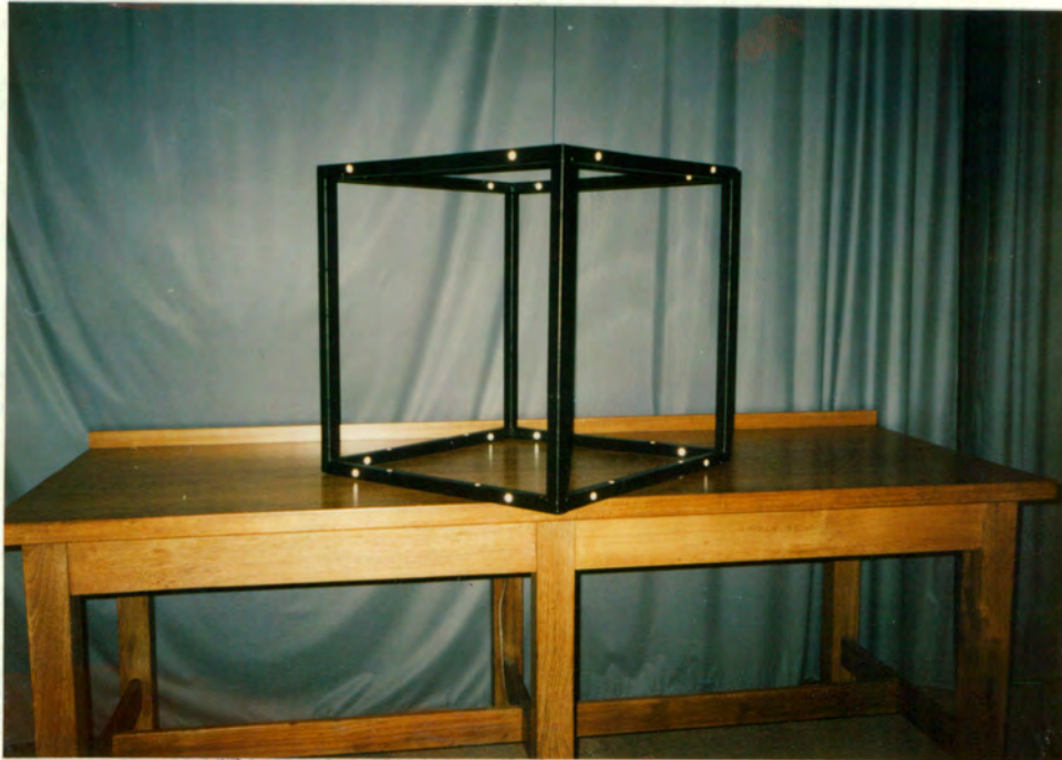
Figure 6.3. Test control frame with targets
