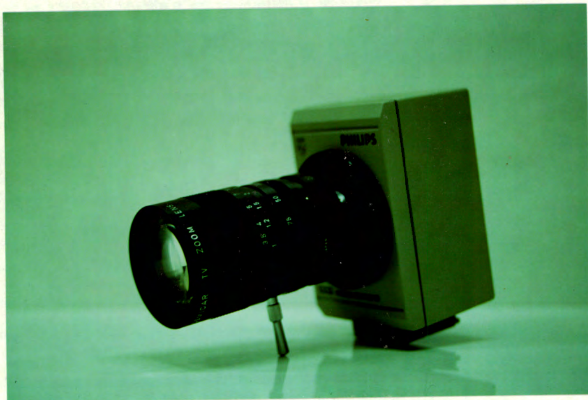
Figure 3.2. CCD camera with telephoto zoom lens
