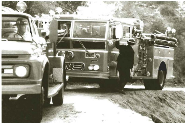
Figure 81: Showing fire truck that is designed for urban use, not suitable and too wide for the roads in the steep wild and urban interface (WUI) (Rice & Davis, 1991).
