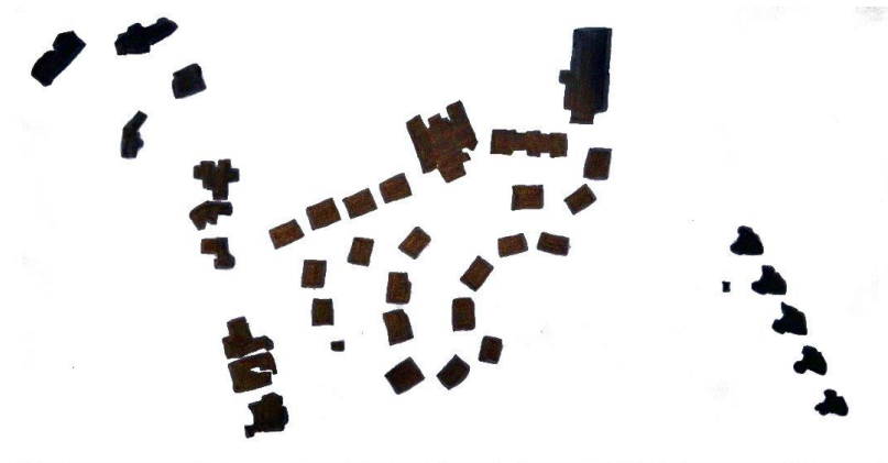
Figure 48: Figure ground showing the Pezula high fire risk dispersed urban layout, note that there is no clustering or defensible space is present (Author, 2022).
