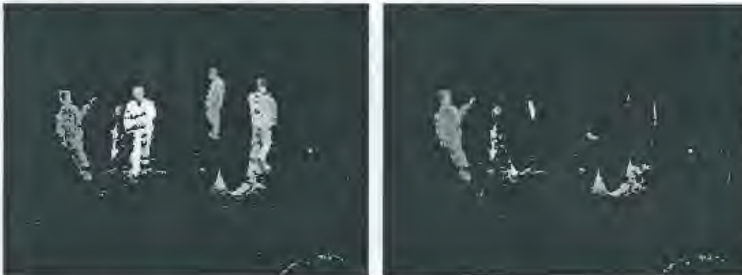
(c) Foreground model after closest target is masked out. (d) Foreground model after all 4 tracked subjects are masked out.
