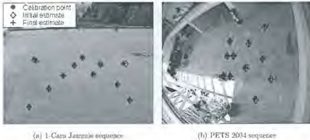
Figure 4.9: Calibration using Tsai's calibration method that makes use of coplanar calibration points.
