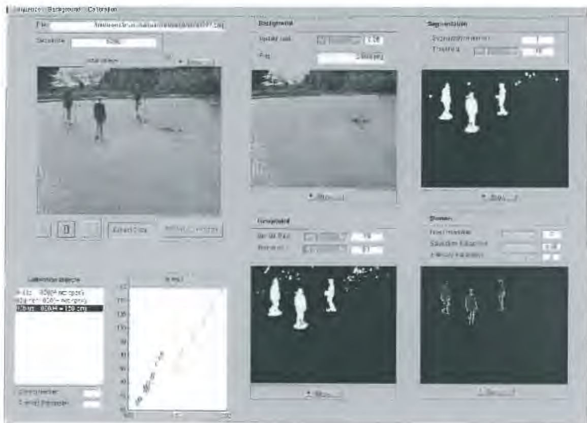
Figure 4.4: Operator interface for the blob tracker. The top left window shows the latest received image and 3 tracked targets and their bounding boxes. The window below shows the (h, i) data that was collected. The other 4 windows show (clockwise from top-left): the current background image, the foreground regions with shadow, the foreground regions with shadows masked out and foreground regions (including shadow regions) that will be masked out in the background update process.
