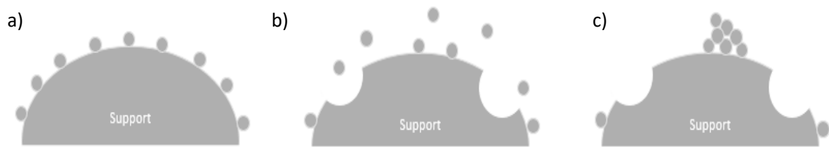
Figure 2.4: Diagram of catalyst nanoparticles and support material for a) the ideal Pt dispersion on the support material b) Pt dissolution resulting from support corrosion and c) Ostwald ripening via Pt agglomeration on a corroded support.
