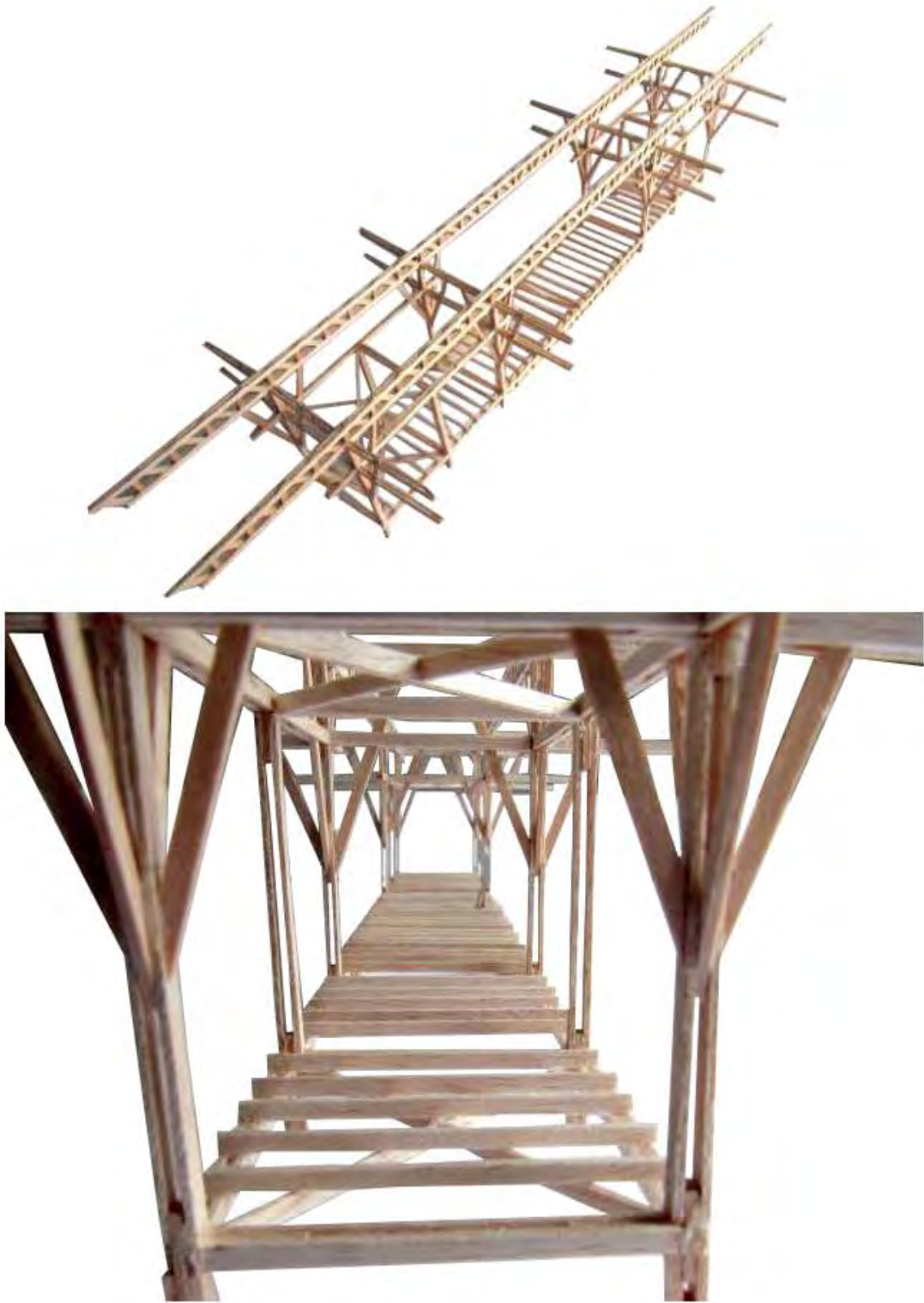
fig. 90 Structural exploration with a span to depth ratio of 1:15. A more elegant structural option
