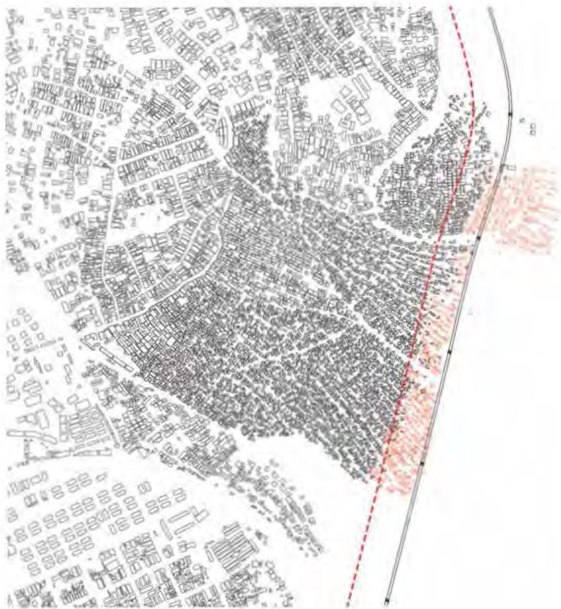
fig. 39 Red dash showing building limitation as a result of high voltage powerlines. The Lagos government demolished dwellings within the 100 meter distance from the powerline in 2012 shown in red.
