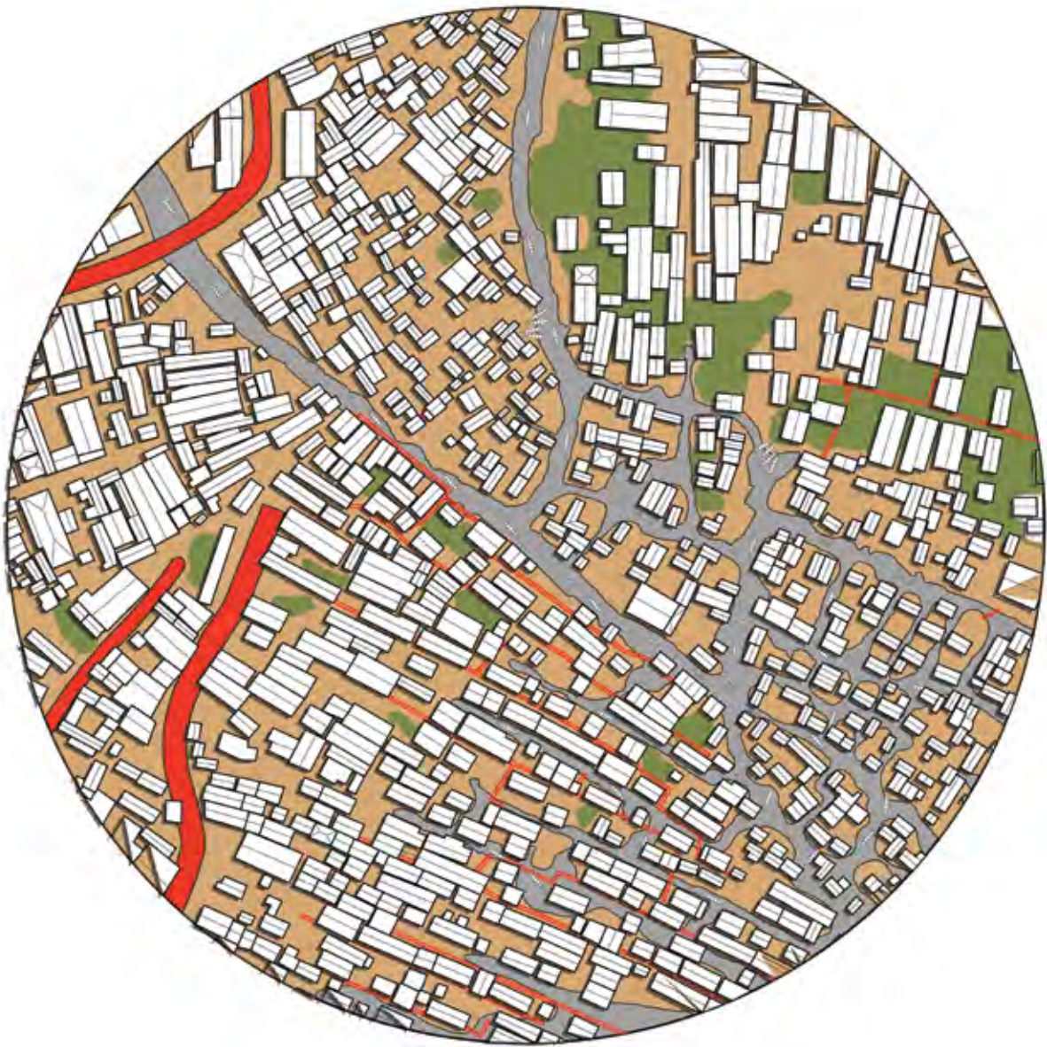
fig. 33 A composite morphological diagram showing the land masses, water routes, pathways and dwellings that form Makoko's urban structure. Study was done at one of the oldest parts of the community.
