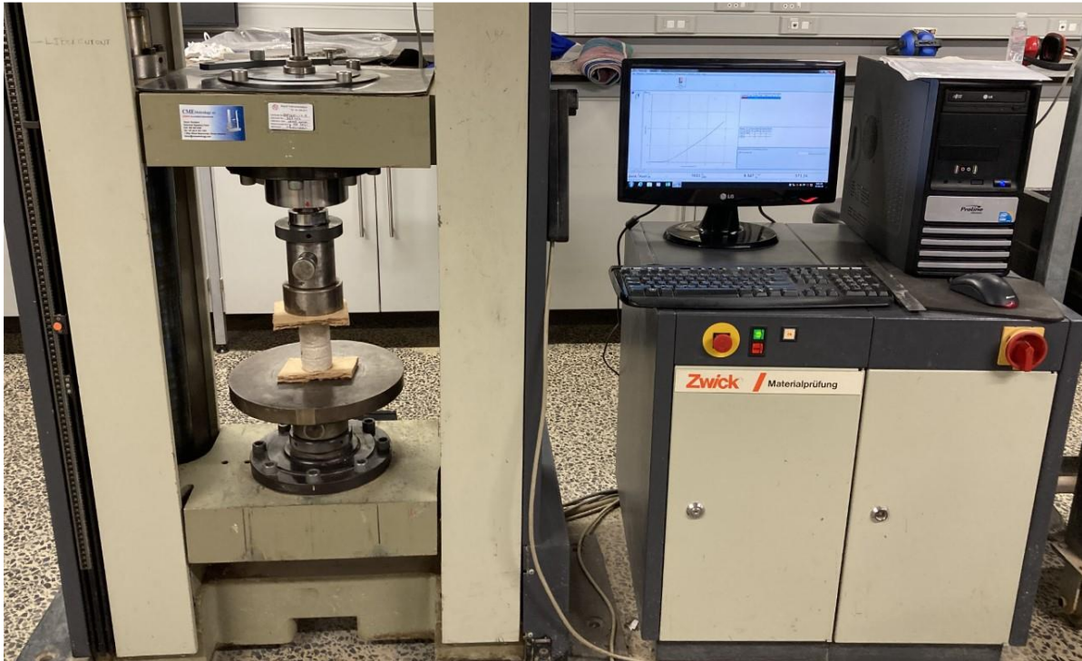
Figure 3.8: Proline Z100 setup used to test the compressive strength each individual bio-column unit. Each unit was placed on the lower bearing and centred beneath the upper bearing which applied a loading force of 100 kN at a rate of 1 mm/min until the unit failed.
