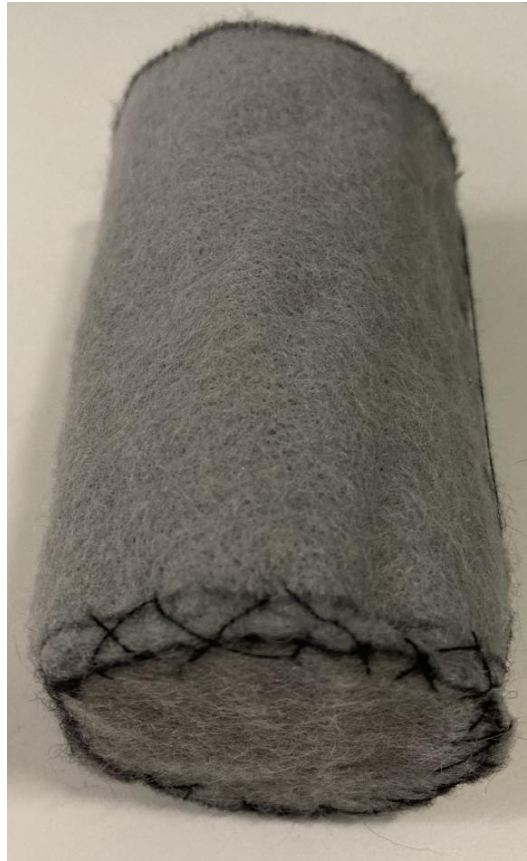
Figure 3.4: Image of geotextile fabric mould used to form bio-columns via the submergent technique. The fabric mould consisted of a 100 mm annular part to which a bottom part of diameter 48 mm was tightly sewn onto.
