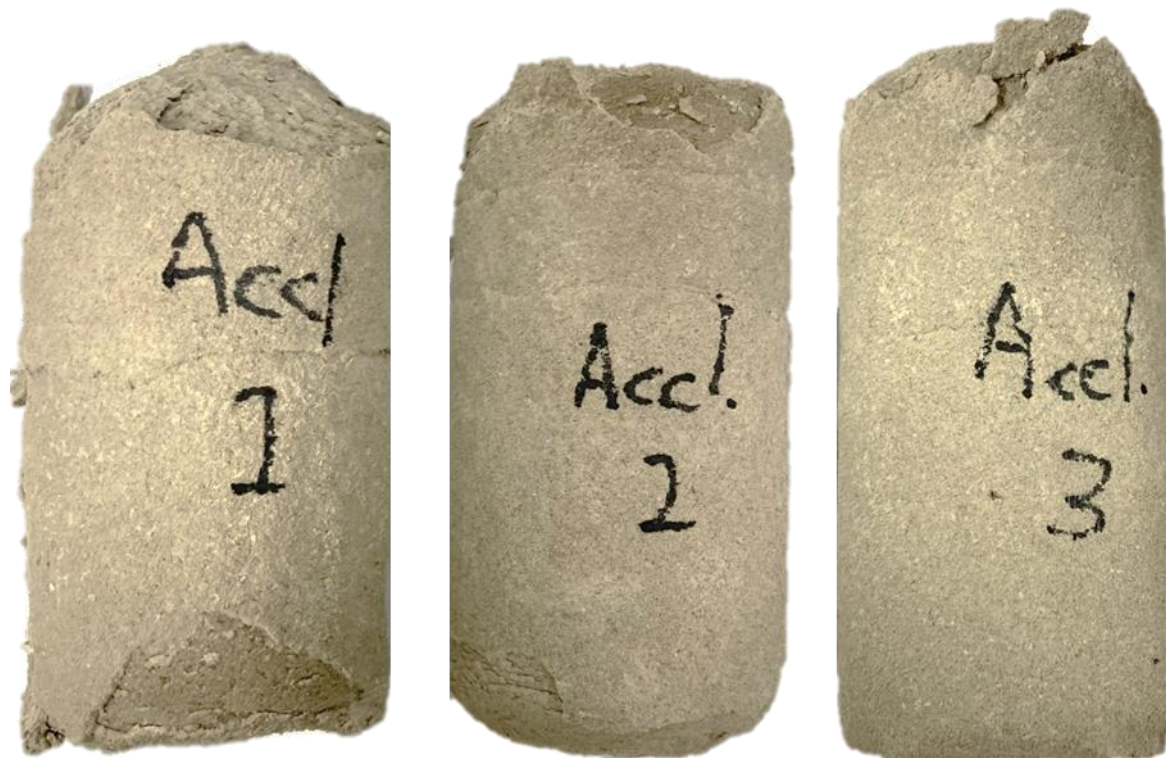
Figure 4.17: Triplicate set of copper mine tailings bio-columns grown using a culture of S. pasteurii acclimatised to 600 mg/L of copper. The bio-columns were brittle, with only one deemed to be suitable to undergo compressive strength testing. Like the previous set of bio-columns utilising copper mine tailings as an aggregate (experiment C), these bio-columns also displayed clear evidence of a shell forming around the outer extremities of each bio-column. However, these shells were slightly thicker and seemed to be of a sturdier nature.
