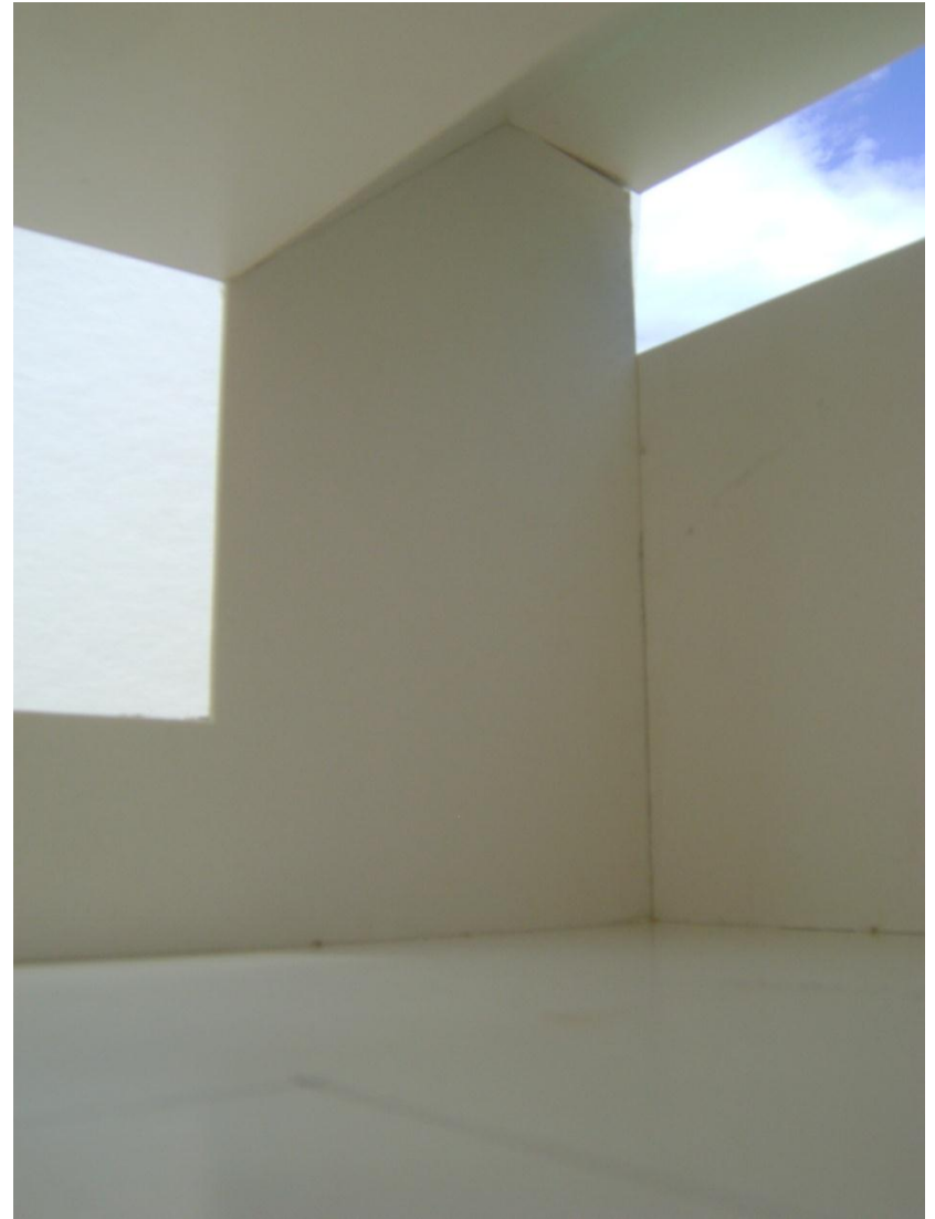
Window with existing white side wall, which reflects more diffused and brighter light into the room
