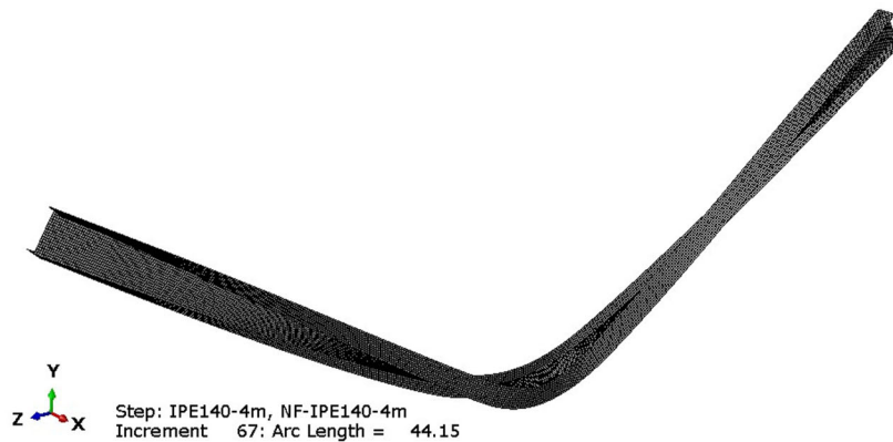
Fig.7-13 A beam failure configuration at a given timestep under nonlinear analysis
