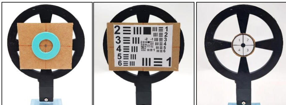
Figure 44: Verification testing targets used for some verification tests. a) Field-of-View test, b) Limiting resolution test, and c) Liquid applicator efficacy test.
