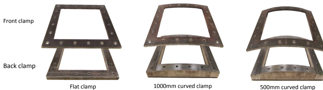
Figure 48: Clamping arrangement for all three panel categories
