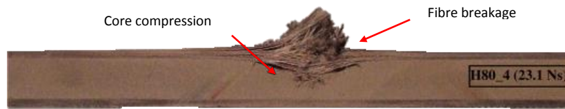
Figure 8: Photograph of a cross-sectioned composite sandwich panel subjected to localised blast load [3]
