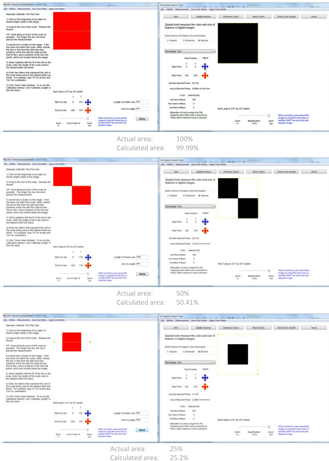
Figure 109: Validation of the calculated delaminated areas: (a) 100% (b) 50%, (c) 25%
