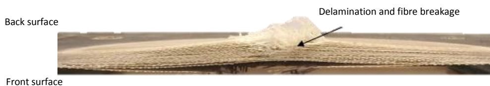
Figure 18: Photograph of a midpoint cross section of glass fibre reinforced vinyl ester panel subjected to a blast load generated from a 13.0g PE4 explosive [28]
