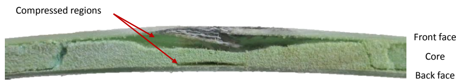
Figure 63: Photograph of a midpoint cross section of a 1000mm FRP sandwich panel subjected to a charge mass of 15g illustrating the compression of the core material
