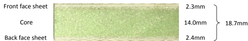
Figure 39: Photograph of a section of the flat FRP sandwich panel, illustrating the effective thicknesses and overall thickness
