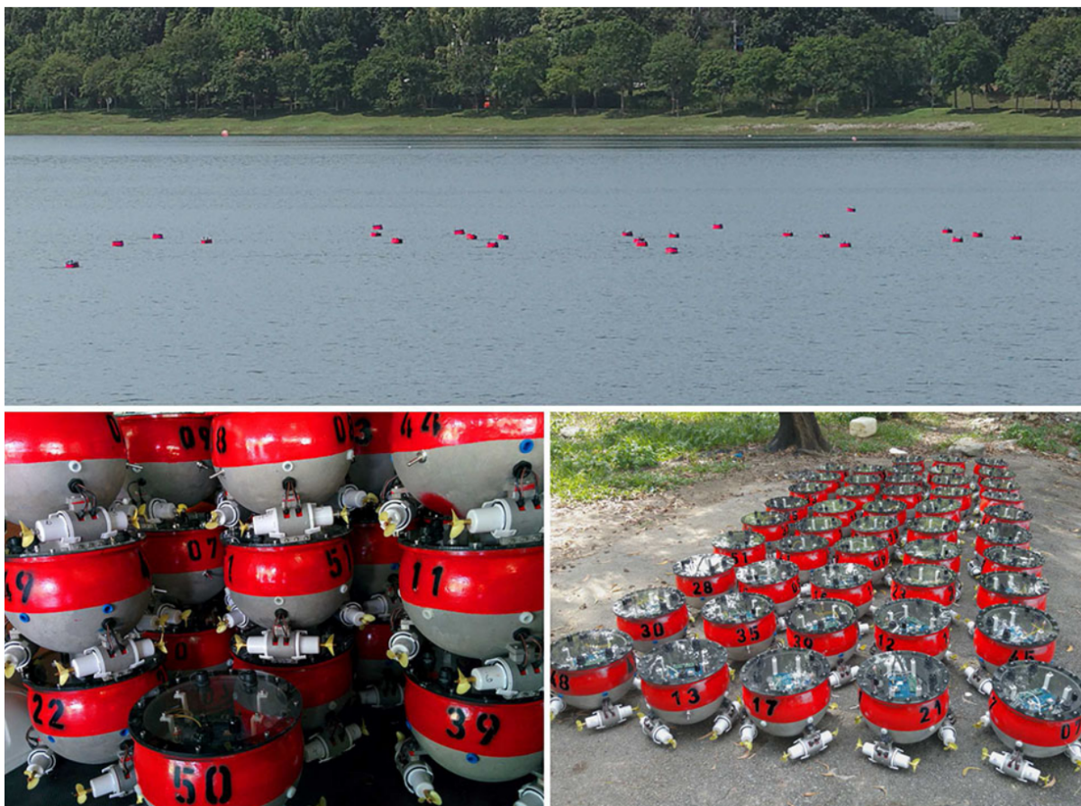
Figure 2.6: Top panel: a swarm of bouys collectively operating. Bottom left panel: a swarm of bouys during transportation. Bottom right: a swarm of bouys just before deployment (Zoss et al., 2018).
