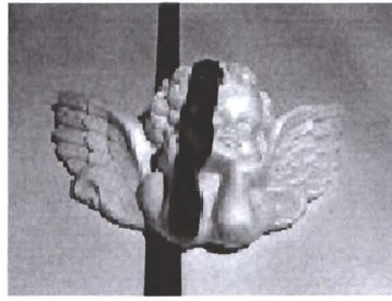
Figure 2.14: Technique for shadow reconstruction (Bouguet, 1999).
