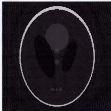
Figure 42: Reconstruction of original head phantom using sparse angle back projection.
