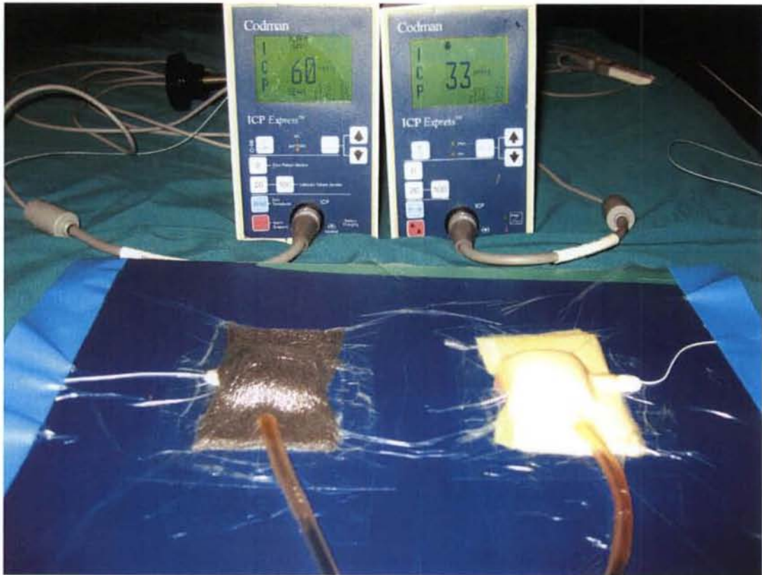
Fig. 34: Cubes of process meat covered by different foams (black reticulated, open-cell polyurethane foam (Kinetic Concepts, Inc., San Antonio, TX, USA) and generic foam) of identical size. Note the greater pressure increase in the meat covered by the polyurethane foam during application of equivalent suction pressures.
