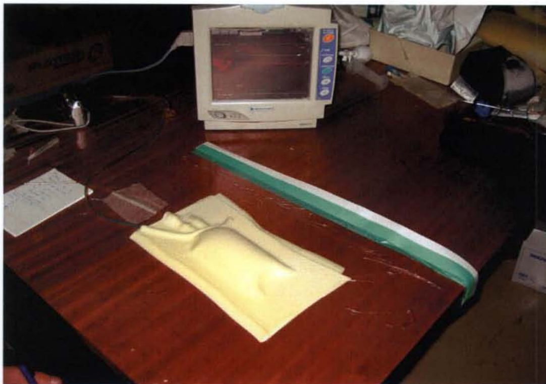
Fig. 6: Non-circumferential NPWT applied over a 50-ml infusion bag. An arterial pressure transducer measures the pressure within the bag.
