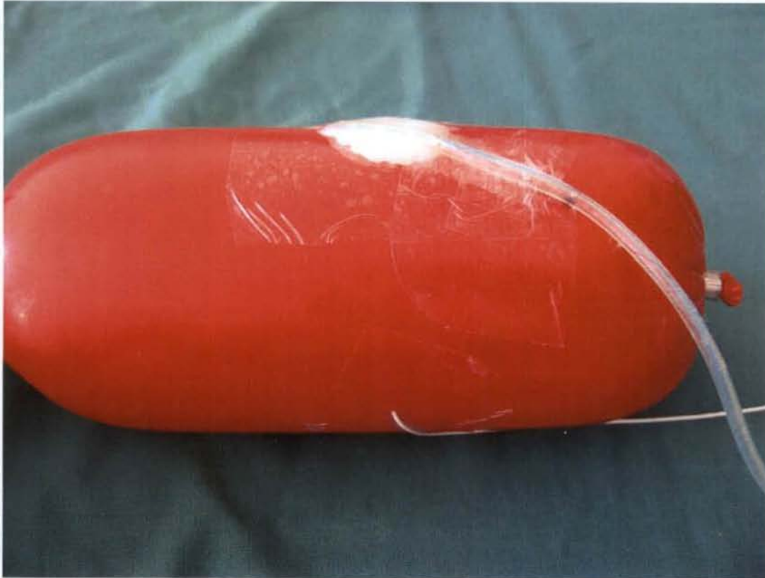
Fig. 53: Processed meat with NPWT dressing inside cavity. Pressure transducer introduced from opposite side and lodged about 1 cm deep to base of cavity.
