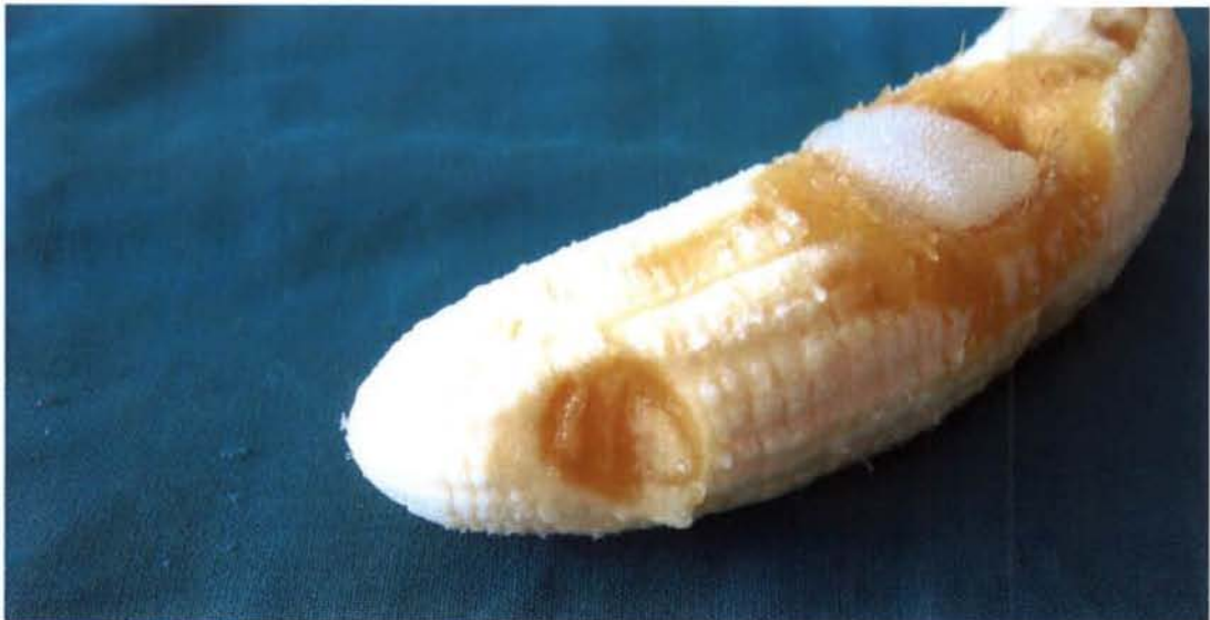
Fig. 17: Flesh of banana demonstrating area of increased pressure surrounding cavity, corresponding to area initially recorded as having increased tissue pressure. The small circle of discolouration at the proximal end of the banana is due to a manual indentation, which was done to observe the effect that external force will have on the banana tissue. Sensor puncture sites are also discoloured.
