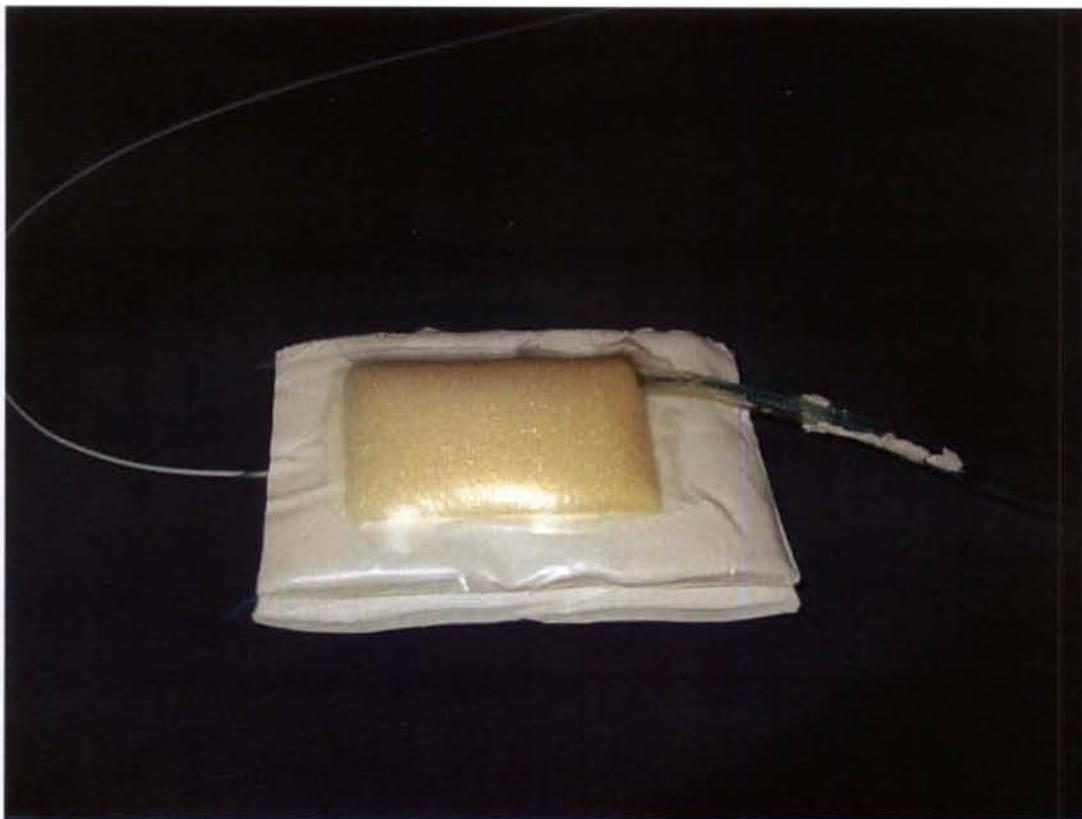
Fig. 11: Sensor between two slabs of Plasticine with NPWT dressing in place.
