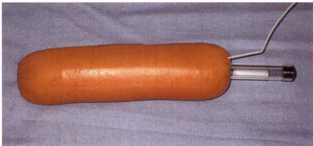
Fig. 50: Sausage skewered onto disposable pen to represent limb/finger with underlying bone. Pressure transducer inserted to a depth of about 5 cm into substance of sausage.
