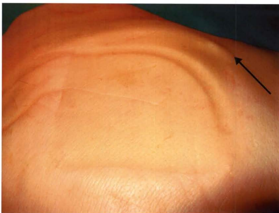
Fig. 22: Impressions left on pork skin by sensor, foam and suction tube (despite tube being laid between two slabs of foam), indicating downward force (vertical force) applied by NPWT dressing. Notice the skin fold (arrow) due to the skin being pulled toward the dressing during foam contraction, indicating the additional horizontal forces that occur.
