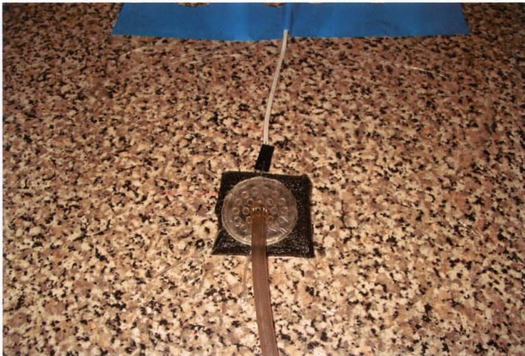
Fig. 36: NPWT dressing square with force sensor beneath it during application of suction.
