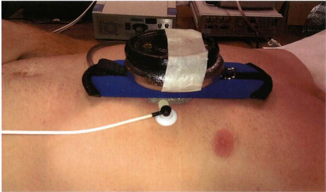
Fig. 92: Photograph illustrating the neoprene band to balance the 1.75 kg weights on the NPWT dressing. Note that no pressure is being applied directly to the sensor.
