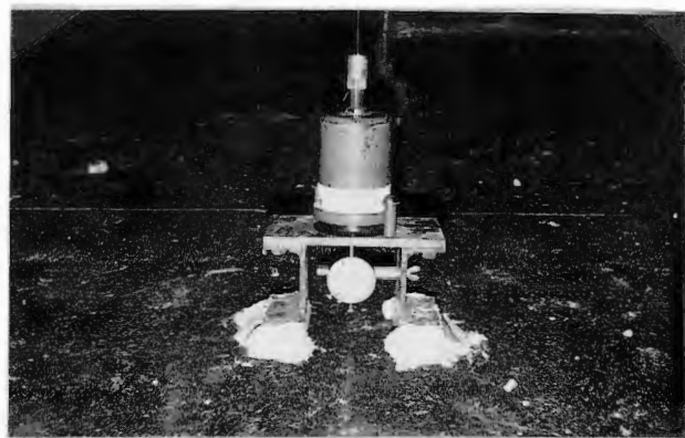
Fig. 6. Displacement gauge bedded on lower deck of portal
