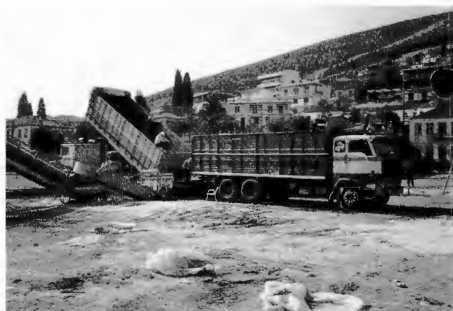
Fig. 2: Lorry tipping Manutube unit for ship loading
