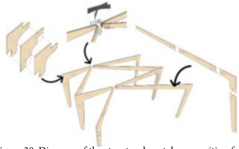
Figure 38: Diagram of the structural portal composition for the dining hall.
