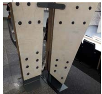
Figure 46: Plywood portal frames footing.
