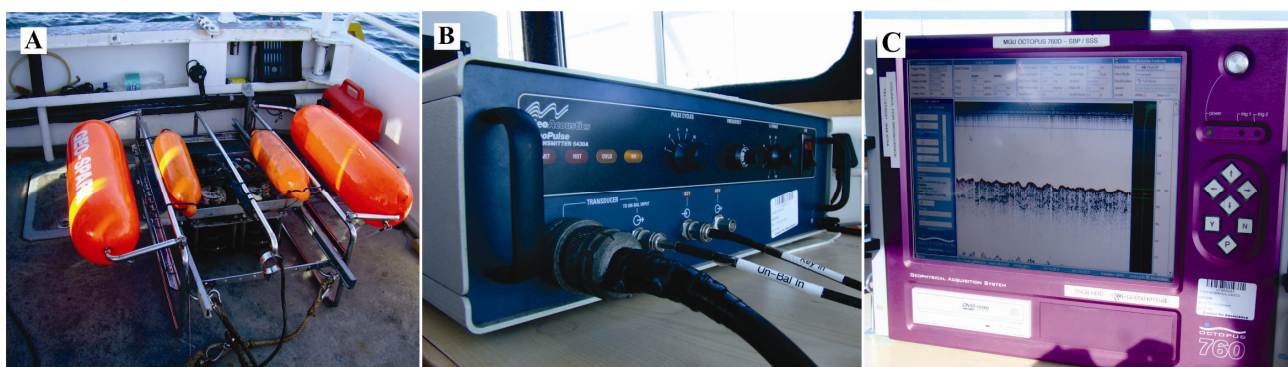
Figure 3-6. Components of the pinger sub-bottom profiling system. A. Massa array transducers in float. B. GeoAcoustics signal transmitter. C. Coda Octopus 760 (topside receiver).
