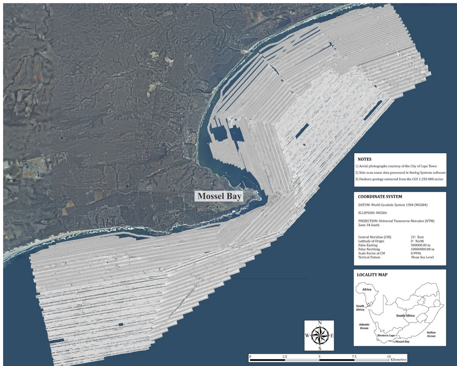
Figure 3-5. Composite side-scan sonar mosaic for the Mossel Bay area. The lines are individual processed tracks.
