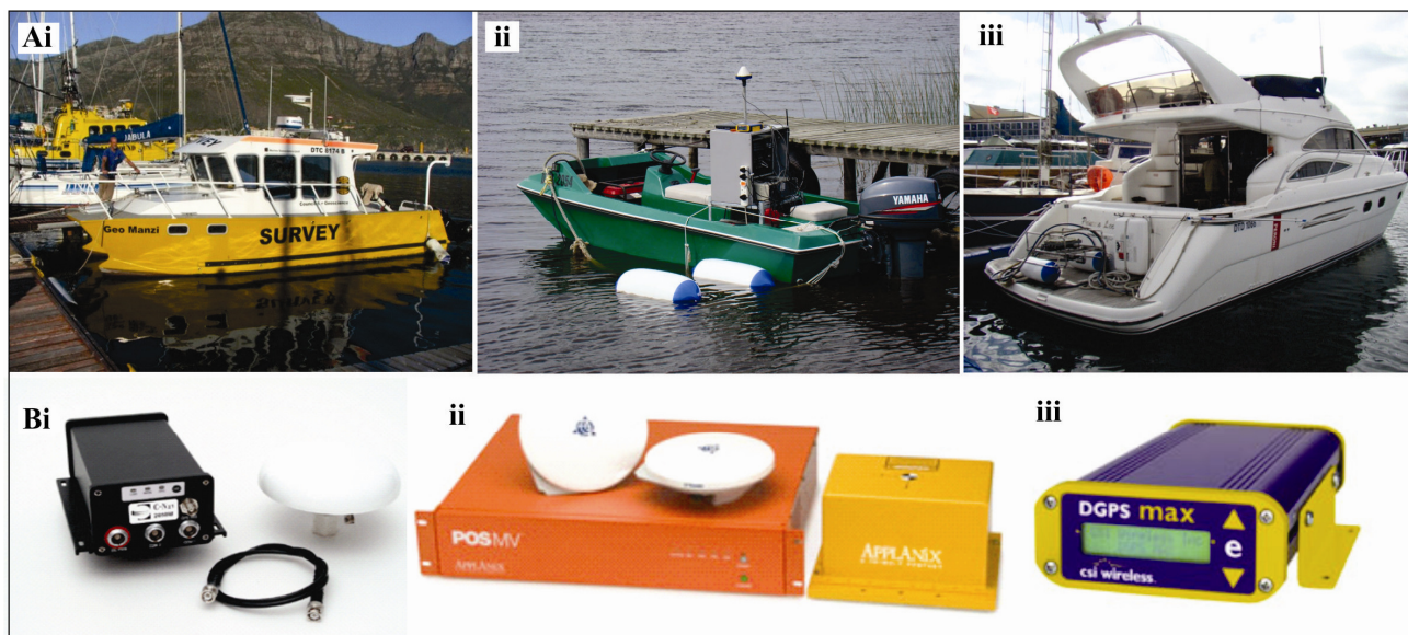
Figure 3-2. A. Vessels used. i. The CGS inshore survey vessel S/V Geo Manzi used for Mossel Bay surveys. Photograph taken in Hout Bay by Dr John Rogers. ii. SAN Parks vessel used in the Swartvlei survey. iii. Vessel M/V Princess Lee used in the regional South Coast survey. B. i. C-Nav 2050 RTG system ii: Applanix POS MV inertial motion reference unit. iii. CSI Wireless dGPS Max navigational system.
